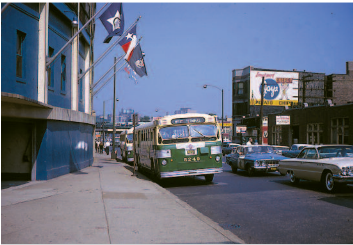
This 52S2P Twin Coach operated in Chicago where propane and trolley buses reduced pollution for many years. The location is Wrigley Field (Cubs Park) at Addison and Clark on Chicago's north side.
