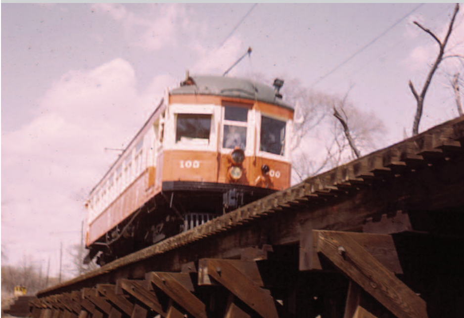
Early interurban cars were built of wood, but most could run at fairly high speeds. They brought mobility to rural areas by letting salesmen cover several towns in one day and by making it possible for rural residents to go to the city to shop yet return the same day. This particular car operated in Iowa.
