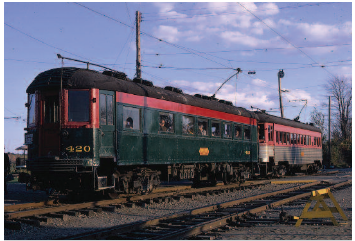
Later interurban cars were made of steel. These cars operated on a line from Chicago to Milwaukee at high speeds and also provided commuter service to numerous locations in the northern suburbs.
