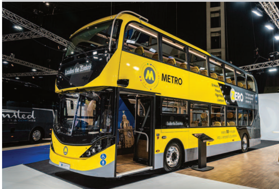
Alexander Dennis unveiled their new hydrogen fuel cell bus at the Euro Bus Expo in early November. This new double-deck model is known as the Enviro400FCEV. Also shown at this event was the battery-electric Enviro 100EV with its next generation electric drive.
