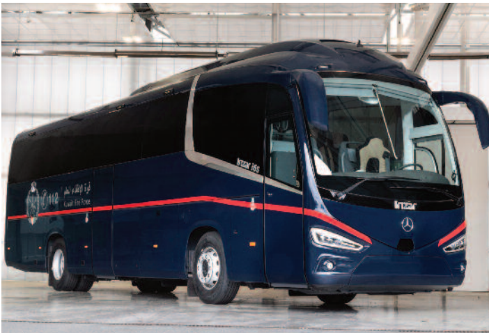
The new premium coach for the Kuwait Fire Force is built in an Irizar 12.2-meter i6S model. This is similar to the popular i6 model sold in the United States but comes with only two axles.
