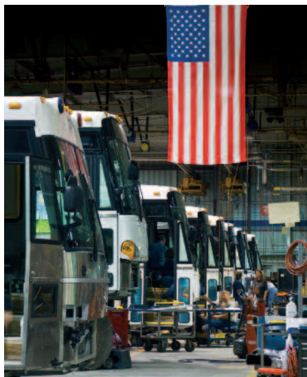
Here is a production line at the facility in Pembina, North Dakota. For decades, the traditional arrangement was that the bus shells were constructed at the Winnipeg facility and then trucked to Pembina for finishing. That first coach on the left is an Inmate Security Transport Vehicle. MCI.
