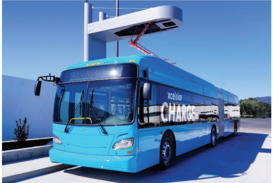
A New Flyer XcelSior CHARGE™ bus is shown being charged from overhead. New Flyer has been building electric buses for generations and is a leader in the field. They offer both conventional size buses as well as the articulated shown here. NEW FLYER.
