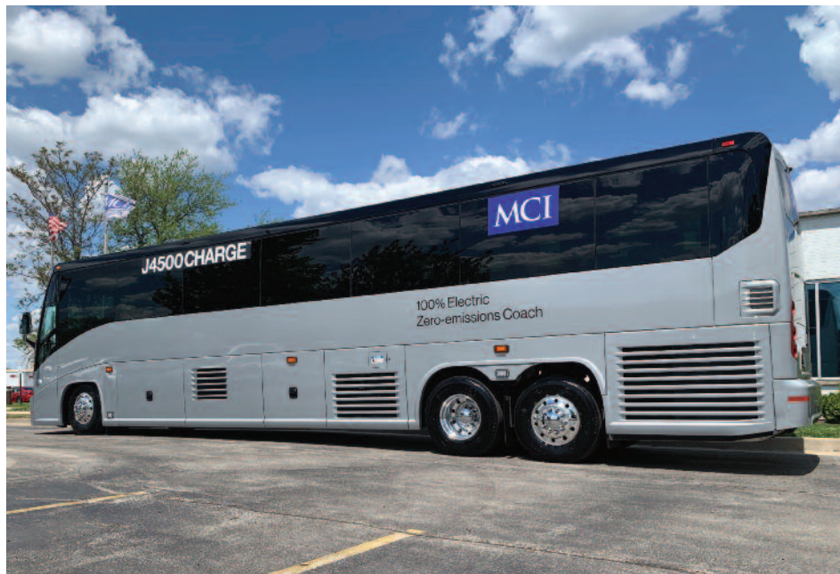
Yankee Line recently operated an MCI battery-electric CHARGE coach in shuttle service at the 2022 US Open. The 52-seat coach operated a full 15-hour shift with a single charge each day. It shuttled attendees between the MBTA Forest Hills station and the Country Club in Brookline, Massachusetts.
