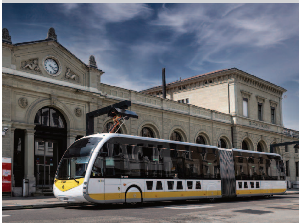
The Irizar ultra-fast charging system in the Swiss City of Schaffhausen was installed a year ago. Fifteen Irizar battery-electric ie tram buses have operated more than 750,000 kilometers and have completed more than 60,000 ultra-fast charging procedures. This proves that a system like this is very workable.
