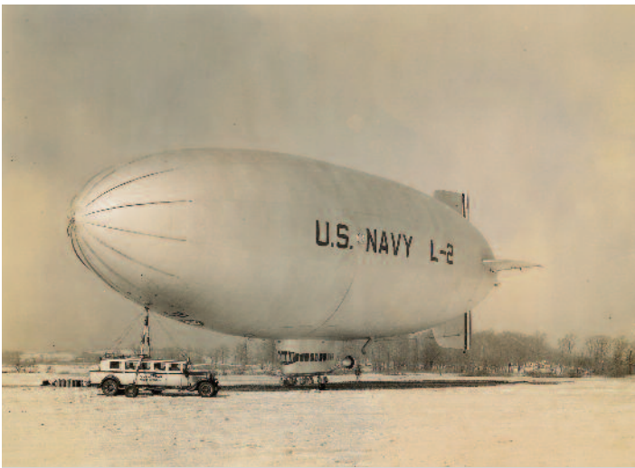
Buses have been used as mobile blimp docks over the years. They help a great deal when docking blimps at places with no regular facilities. Shown here is an early Flexible bus used by Goodyear as a blimp dock. NBT ARCHIVES.
