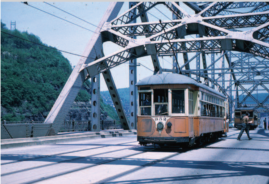
In the early days, streetcars carried the bulk of transit riders. However, Americans fell in love with their new automobiles and they soon took over as the most popular means of local transportation. Shown here are a pair of streetcars crossing the Franklin Bridge in Johnstown, Pennsylvania. Note that a second overhead wire is already in place for replacement trolley buses. NBT ARCHIVES.
