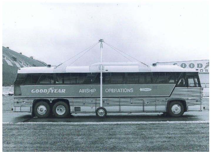
In later years, Goodyear moved to using newer models of buses as mobile blimp docks. Shown here is an MC-8 used for this purpose. The buses also helped blimp operations by carrying supplies and spare parts. NBT ARCHIVES.
