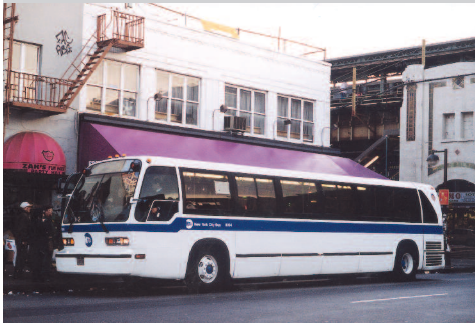
The General Motors modular RTS (Rapid Transit Series) model was originally planned as a short-term replacement between the "New Look" models and the proposed new TransBus. Since the TransBus never went into production, the RTS lingered on for many years as one of the most popular high-floor transit buses before the industry started going to low-floor models. After General Motors sold, MCI acquired this line and moved production to Roswell, New Mexico. This example was photographed in Brooklyn, New York on January 1, 2000. J.C. REBIS JR.
