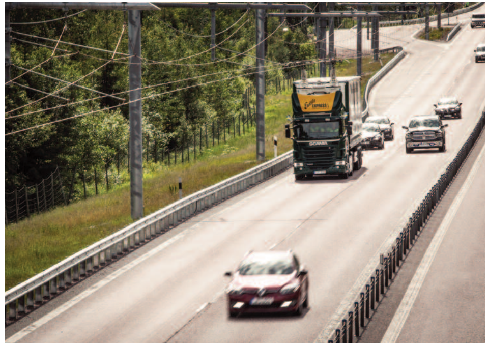
This photo was taken on the first eHighway installation in Sweden. It originally opened in June of 2016 on a stretch of highway north of Stockholm. Scania trucks used to test the highway are powered by bio-diesel hybrid systems so they can easily operate off the eHighway system.
