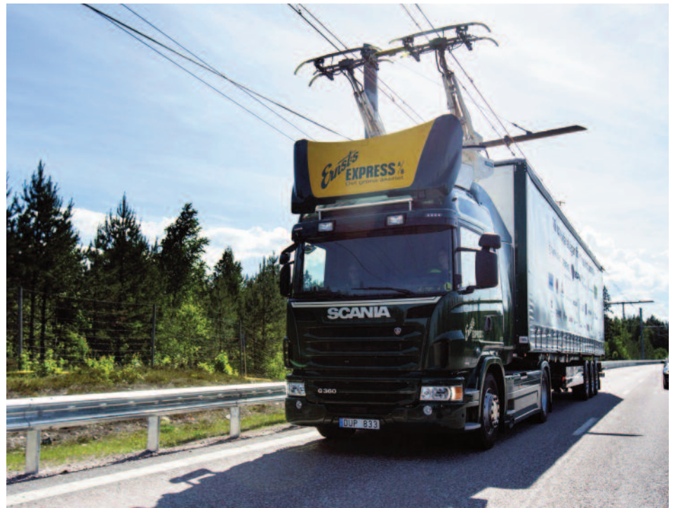
No lane guidance system is required since the intelligent pantograph system will automatically extend up to the wires to connect and will also disconnect automatically if the vehicle makes an abrupt maneuver or changes lanes.
