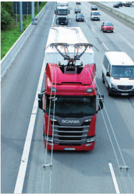
Vehicles using the system are equipped with a modified pantograph current collection device that can pick up both positive and negative current from both sets of wires. The voltage in the wires is similar to that used by trolley cars and trolley buses.
