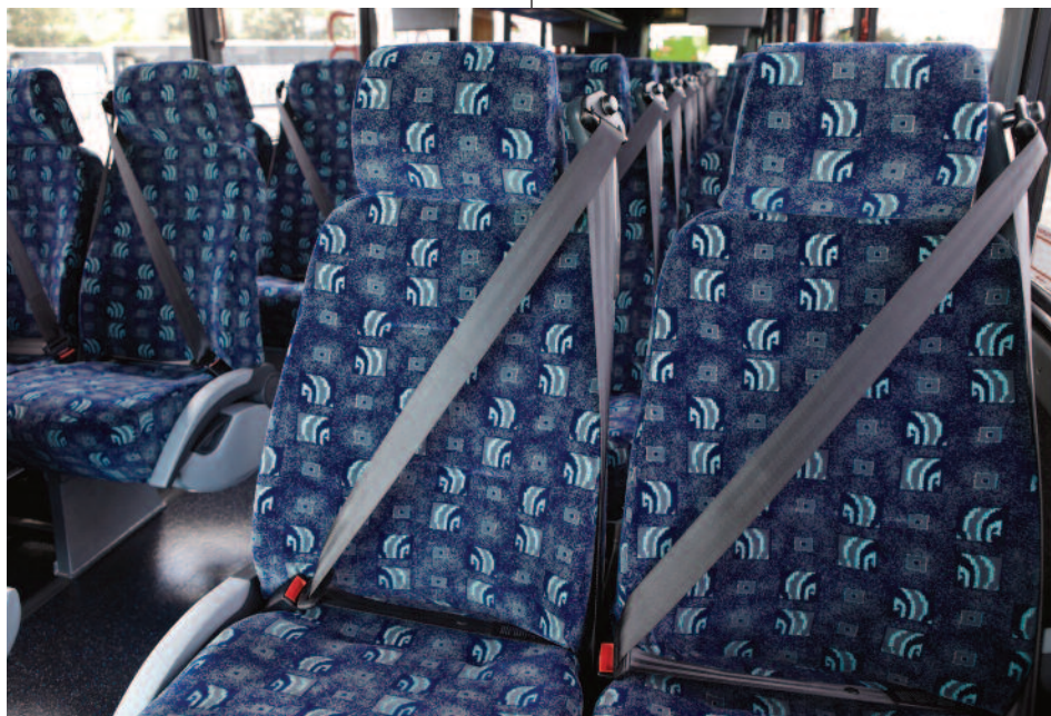
Some people in the bus industry still debate the relative value of compartmentalization and seat belts. The mandate for seat belts came from regulators trying to do something following an accident and not from a long and detailed study. Shown here are Amaya seats with seat belts installed on a Van Hool coach. ABC COMPANIES.
