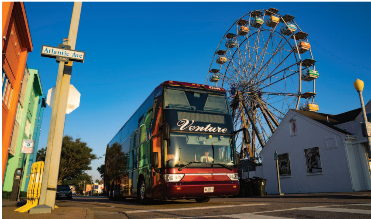
Double-deck coaches can bring a crowd to your location since they can seat as many as 80 passengers. You must have sufficient overhead clearance since these coaches are 13 feet tall. All buses require suitable roadways with gentle turns and a lack of obstructions. VENTURE TOURS.
