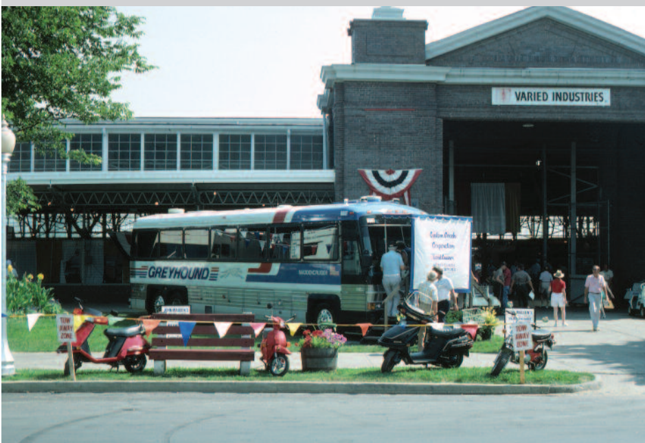
The first Madden Cruiser resulted from a three-year contract with Greyhound. The resulting coach was an MCI 102A3 painted in Greyhound colors and carried fleet number 0001. It was photographed while on display at the spring 1987 FMCA event. NBT.
