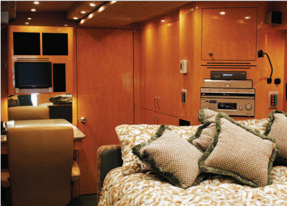
Shown here is the rear of Madden Cruiser number five. This coach featured an expanded work area at the left, the large bed on the right and a four-foot by four-foot steam shower. The bed was mounted on sliders and could be moved when not in use to increase the aisle width. MCI.
