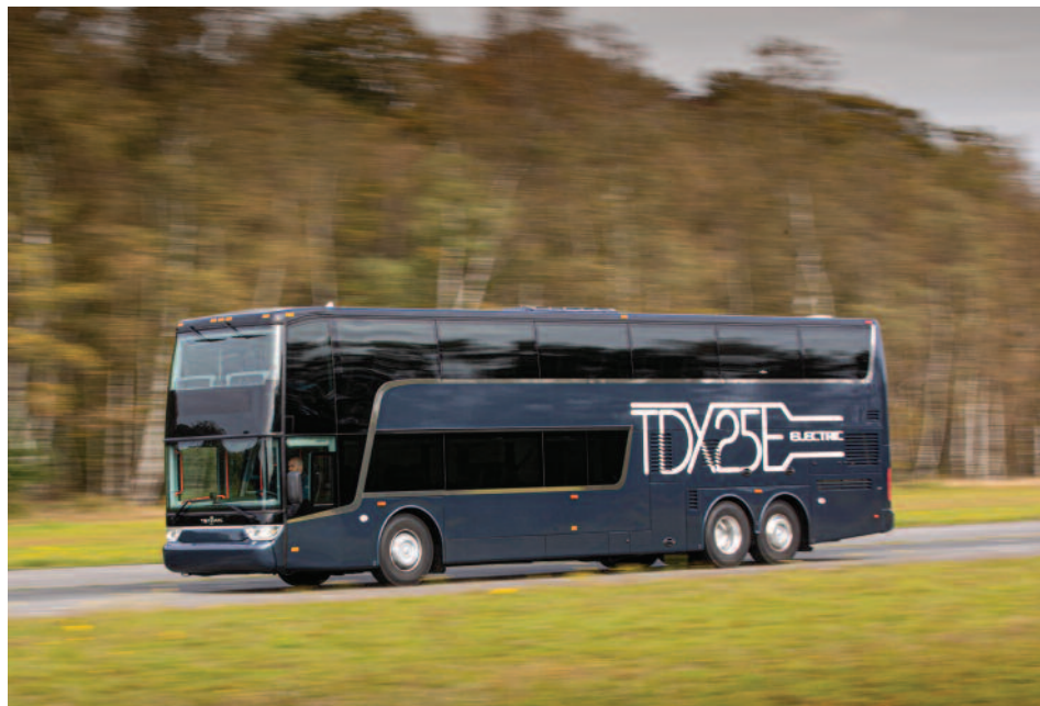
Van Hool recently introduced the first battery-electric double-deck coach. It combines the electric battery power technology of its existing single-deck Van Hool CX45E coach with its popular double-deck model to create the battery-electric TDX25E model. This new model will seat 69 passengers with 18 on the lower deck and 51 on the upper deck.
