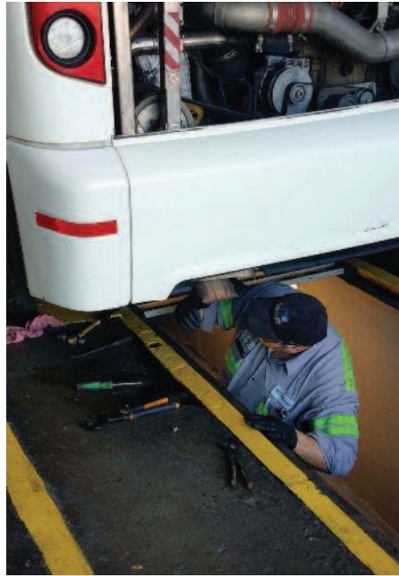
Trans-Bridge Lines devotes substantial space to service and support that includes a wash bay, body shop and a parts department. Shown here is one of the pits for working underneath the buses.
