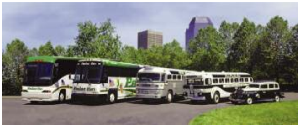
This photo shows the transition in Peter Pan vehicles over the years. Included is the Buick sedan, the GM PD2903, a PD4103 and two newer MCI coaches. Downtown Springfield is in the background.
