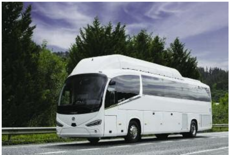
The most recent development that is turning heads is the new i6 hydrogen-powered coach from Irizar. This coach has a range of more than 60 miles and can be refueled in 20 minutes. It can also run as a battery-electric coach for short periods. IRIZAR.
