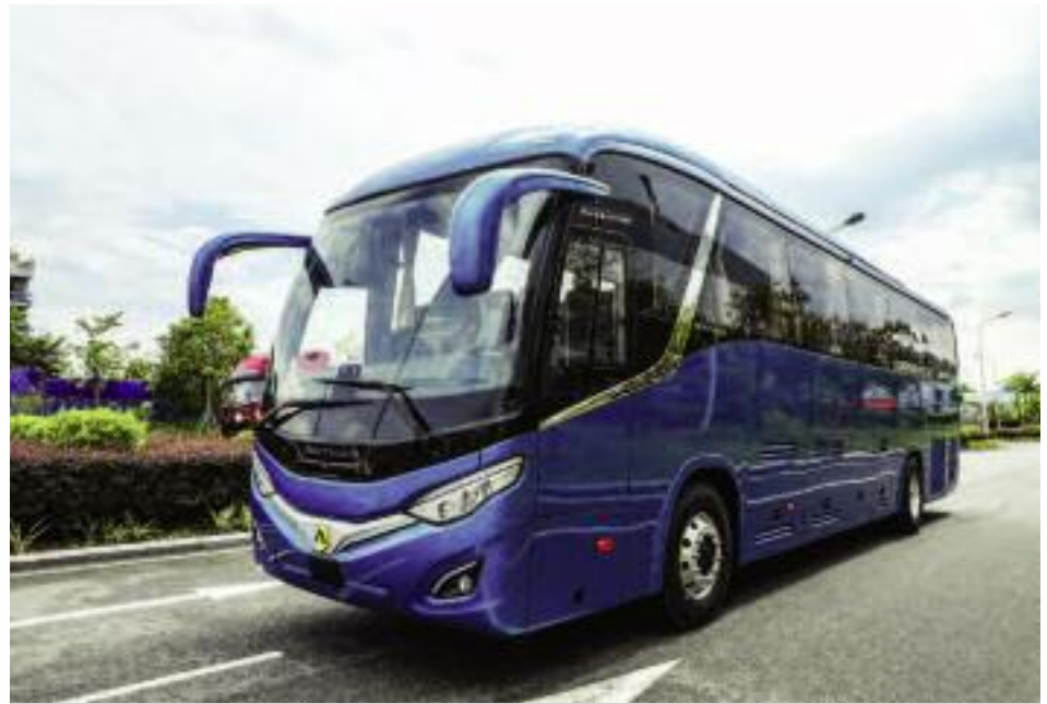
In September of 2022 Marcopolo showed its hydrogen fuel cell bus at the IAA show in Hanover, Germany. It had a length of about 39 feet, seated 53 passengers and came with ZF axles as well as Knorr air suspension and brakes. This early model offered an operating range of about 370 miles. MARCOPOLO.
