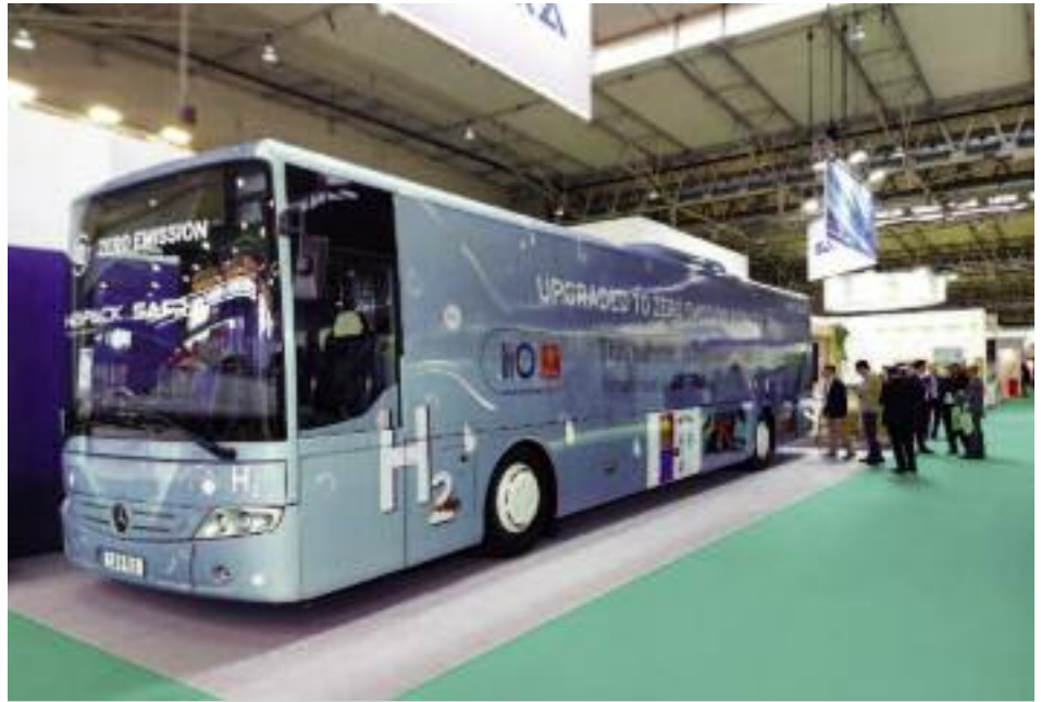
The hydrogen fuel cell industry has progressed to the point where you can actually buy a kit to convert a diesel bus to hydrogen. In early June of 2023, SAFRA from France introduced their H2PACK® hydrogen retrofit kit at the Public Transit Summit in Barcelona. The Mercedes-Benz coach on display is one of 15 that SAFRA was retrofitting with hydrogen power for the Occitanie Region in France. SAFRA.
