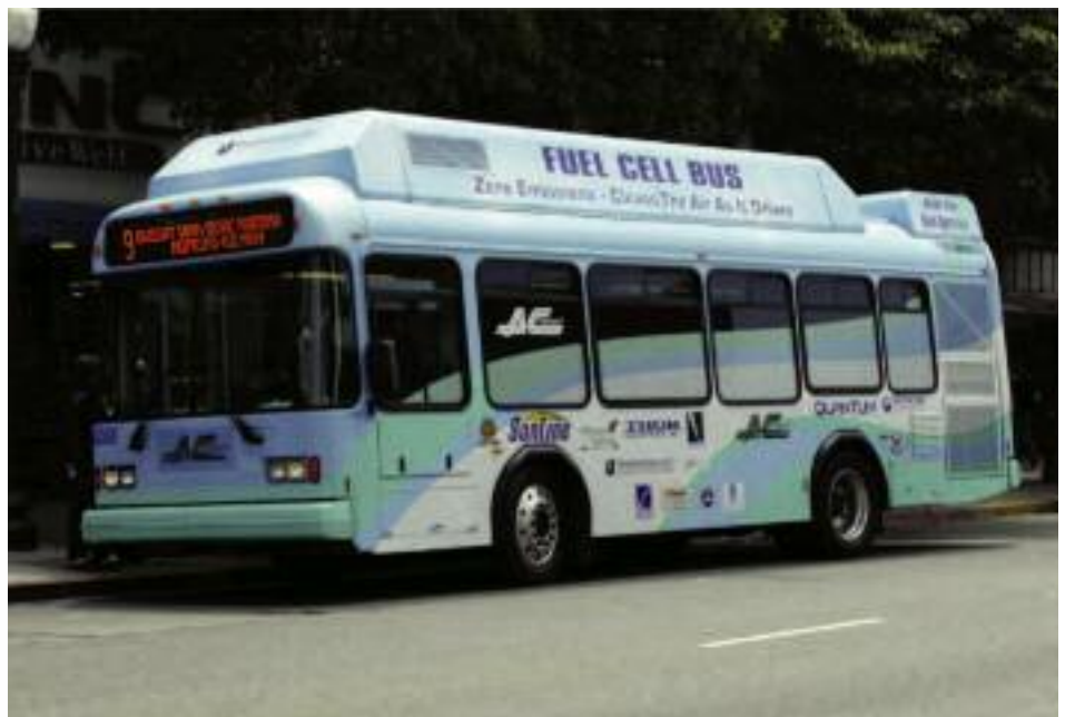
It was the early hydrogen fuel cell transit operation at AC Transit in the East Bay area that showed that hydrogen was practical for bus operations. AC Transit developed its own hydrogen energy station in 2002 and then put their first hydrogen bus in operation in 2003. Shown here is that first hydrogen bus using a bus from Thor Industries, a fuel cell from UTC and power control software ISE. AC TRANSIT.
