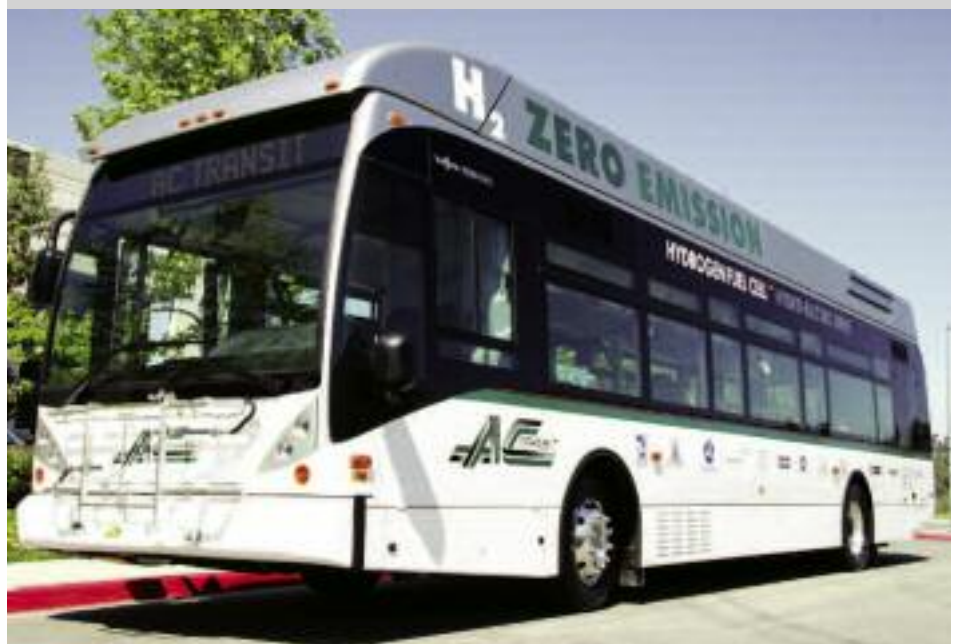
AC Transit acquired three 40-foot A330 buses without engines from Van Hool that were called gliders. They were then equipped with hydrogen fuel cells from UTC, electric motors from Siemens and power controls from ISE. These buses operated successfully in heavy-duty transit service that proved that hydrogen was perfectly capable of becoming a viable alternative fuel. AC TRANSIT.
