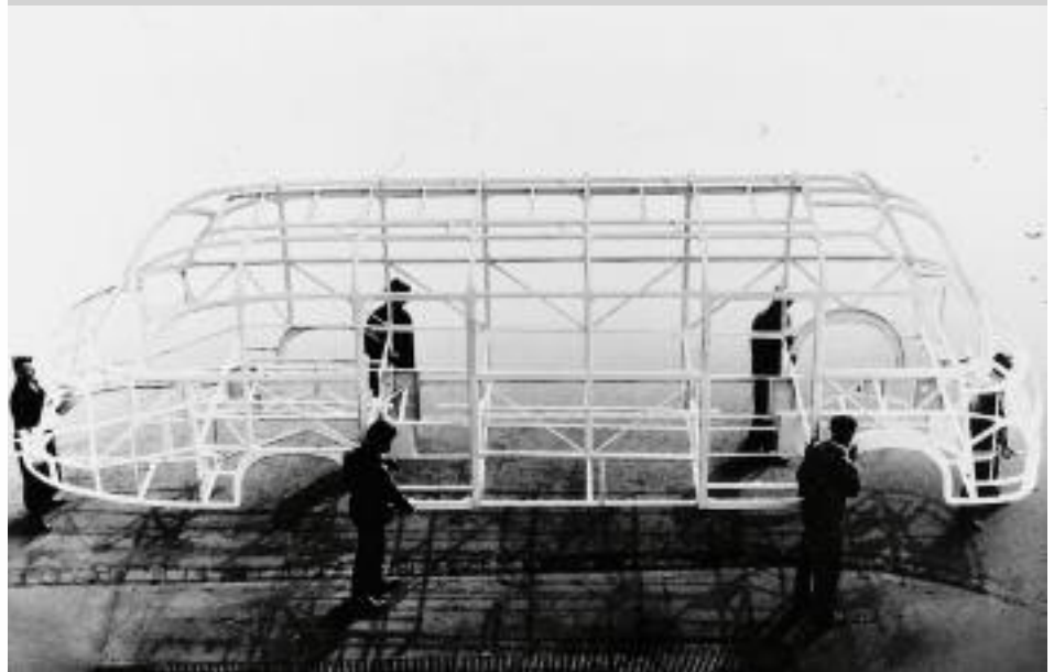
Kässbohrer in Ulm, Germany developed integral construction in 1951 that they called "selbsttragend" or "self-supporting." It was originally used in their short S-8 model and started their Setra line. This historic photo has six Kässbohrer staff members holding the frame structure to show its light weight.
