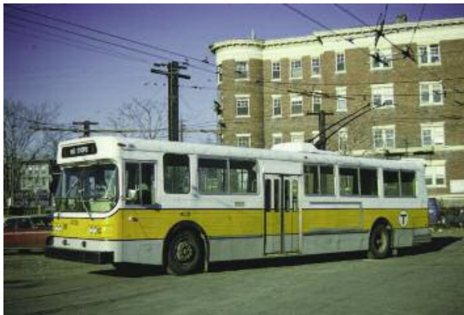
New Flyer was a Canadian pioneer in zero-emission buses and built a large number of trolley buses. Shown here is one of 50 E800 trolley buses that went to Boston. That door on the left side permitted operation at a station platform.
