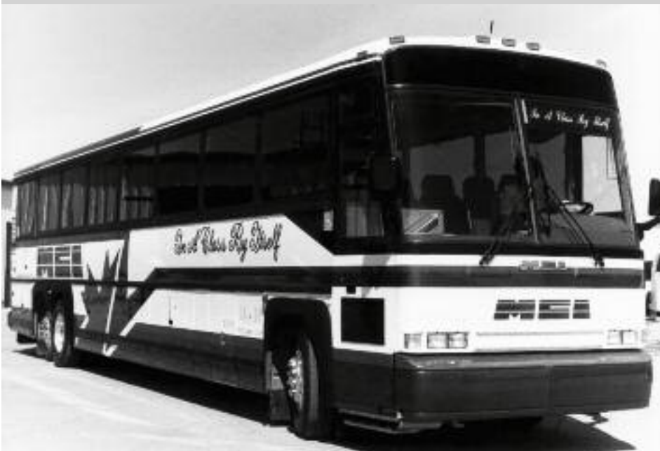
With the 45-foot coach length on the horizon, MCI worked with the Canadian government in 1990 to produce a prototype coach for the disabled in a length of 45 feet. It had several features for the handicapped including a lift for mobility devices and an accessible restroom. While this coach never went into production, it did serve as a prototype for the 102DL3 model that was introduced after the 45-foot length was approved.
