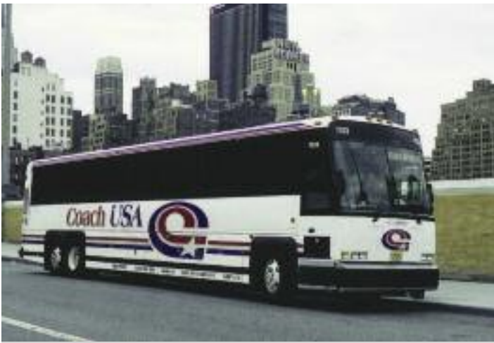
When the 45-foot length was approved, MCI introduced their new 45-foot 102DL3 model at the UBOA Bus Expo in Chicago in February of 1992. It offered the newer Series 60 engine in a larger engine compartment and went on to become MCI's most popular model for several years.
