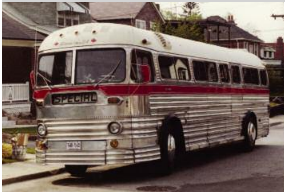
The Courier 95 Model helped establish MCI's reputation for reliability and durability. As was typical of that era, buses imitated the bright siding of passenger trains and the new General Motors coaches. MCI was prone to use stainless steel because it held up well in bad weather.
