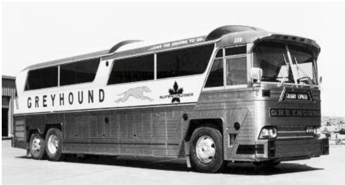
Originally intended to be a replacement for Greyhound's Scenicruisers, the MC-6 model offered several innovations including three roof heights, a 12-cylinder engine and a width of 102 inches. The new width proved to be a problem and only 100 production units were built. This builder's photo shows one of the units that was going to Canada.
