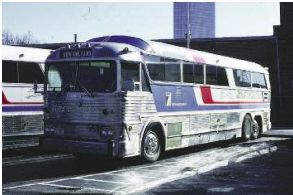
The new Fort Garry plant was established to build the new MC-6 coaches because of their 40-foot length. However, because of delays with the MC-6 model, production at Fort Garry started with the MC-7 model that ended up being the replacement for Greyhound's aging Scenicruiser fleet. Shown here is the first production MC-7, noteworthy because of the partial wheel covering on the third axle. ROBERT REDDEN, REDDEN ARCHIVES.
