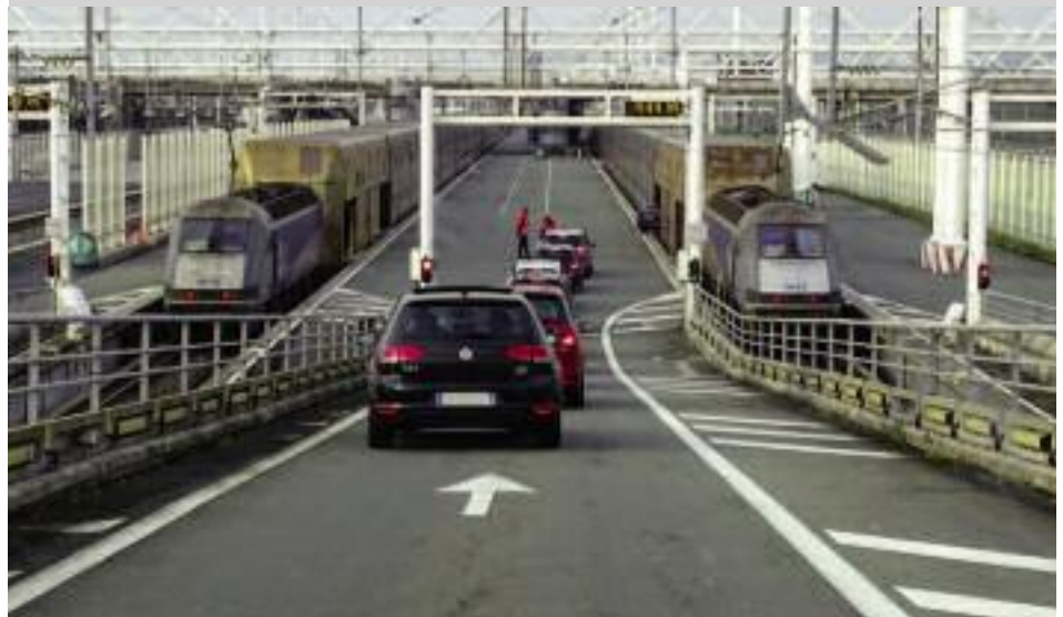
One of the best examples for transporting passengers along with their autos can be seen on the EuroTunnel operation between England and France. Special railroad cars are used that allow the automobiles to be driven inside the train and then off again on the other side of the English Channel. This photo shows automobiles being driven down the ramp leading to a train that is filling up prior to departure. ©AD MESKENS / WIKI-MEDIA.
