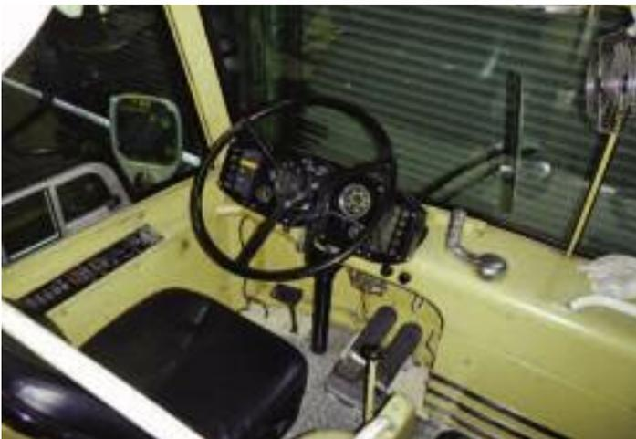
The cockpit area of the Scenicruiser was similar to the PD4104 in using toggle switches and a meaningful side panel. Like the rest of the fleet, the Scenicruiser in the Historical Fleet had been converted to the 8V-71 engine. MICHAUD BUS APPRAISALS.
