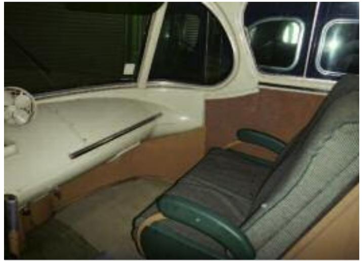
The seat to the right of the driver on the Brills accommodated two passengers. In the center of the dash is the knob for the air-operated control for opening and closing the door. MICHAUD BUS APPRAISALS.
