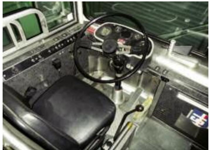
The cockpit area of the MC-7 brings us into a more modern area. This was the last model in the Greyhound fleet with a clutch and mechanical transmission. MICHAUD BUS APPRAISALS.
