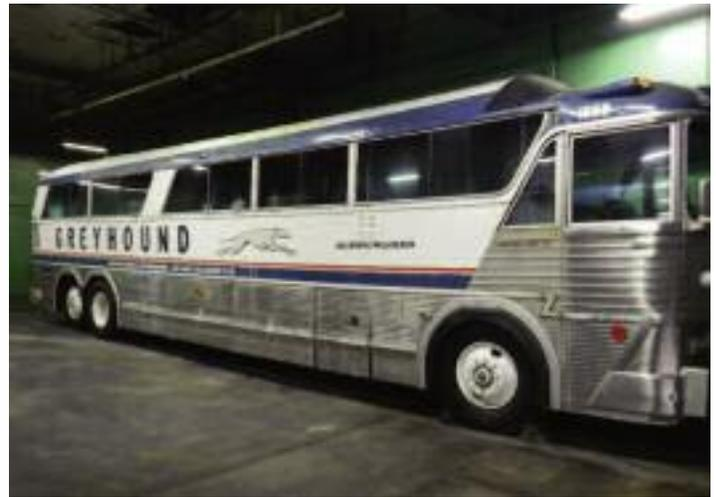
For many of us, the MC-7 moves up into a more modern era. It effectively was an extended and raised MC-5 with a higher passenger level and a length of 40 feet. The MC-7 was the model that effectively replaced the Scenicruiser in the Greyhound fleet. MICHAUD BUS APPRAISALS.
