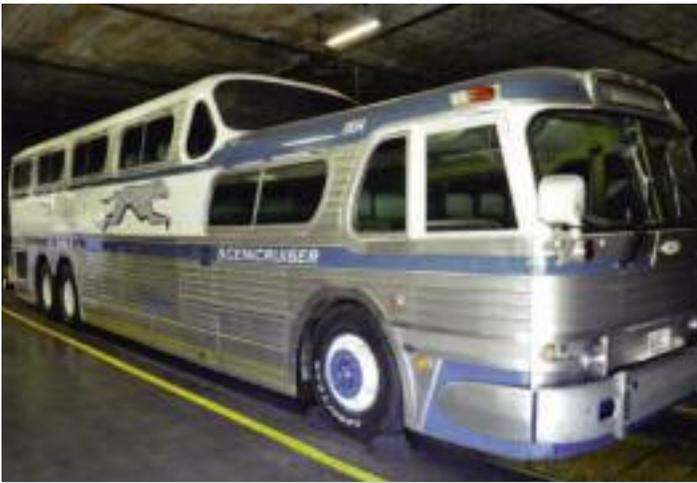
To a large extent, the Scenicruiser represents the queen of the Historical Fleet. It required many years of development and brought the coach industry up to the 40-foot length. Originally built with dual 4-71 diesel engines, the Scenicruisers were later updated to a single 8V-71 engine. MICHAUD BUS APPRAISALS.
