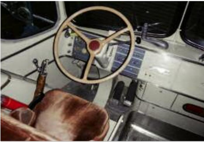
The cockpit area of the Silver Side continued with the push-pull switches on the dash of the previous models. However, its defining feature was the column-mounted shift lever and the air-assist clutch that provided a unique sound in operation. MICHAUD BUS APPRAISALS.
