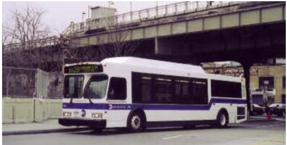
The roofline gives this away as a CNG-powered bus, another move to alternative fuels. It is a 2001 Orion 07 operated by MTA New York City Transit and was photographed on Bedford Park Boulevard in Bronx, New York on January 29, 2002. J.C. REBIS JR.
