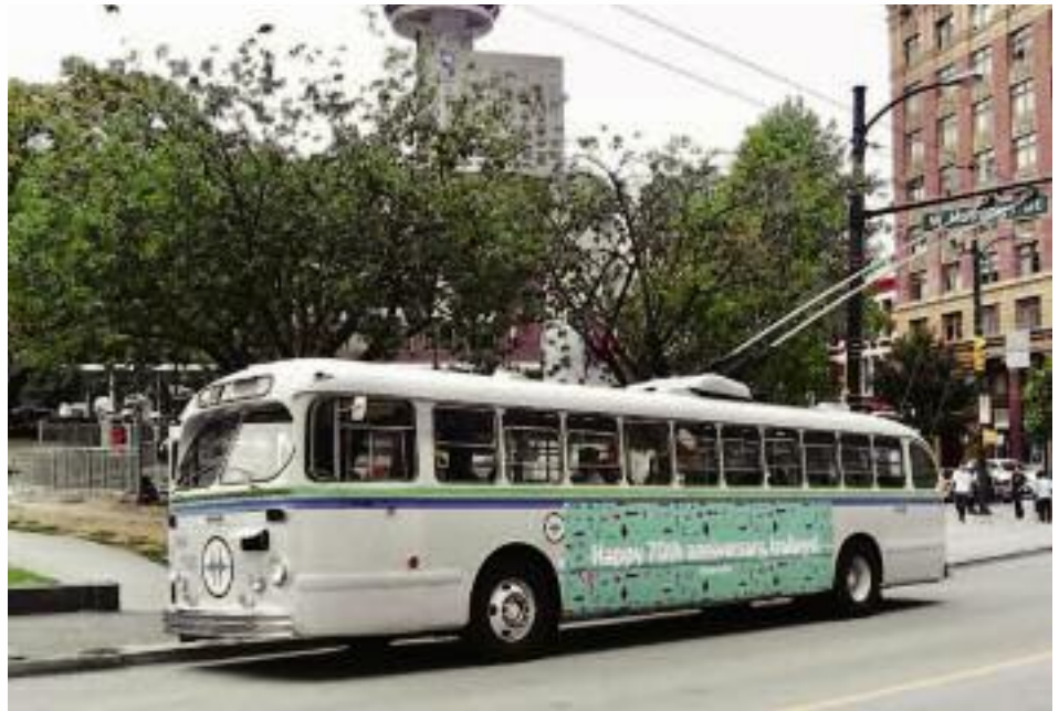
In many cities trolley buses replaced the streetcars. They required two overhead wires but continued to use the same power as the streetcars. Although uncommented at that time, they operated with zero emissions. This Brill trolley bus operated in Vancouver, British Columbia. ANGUS MCINTYRE.
