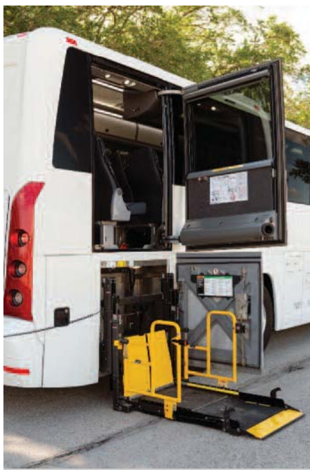
The wheelchair lift on the D4520 is placed at the rear of the coach. This eliminates the need to reduce underfloor luggage space.
