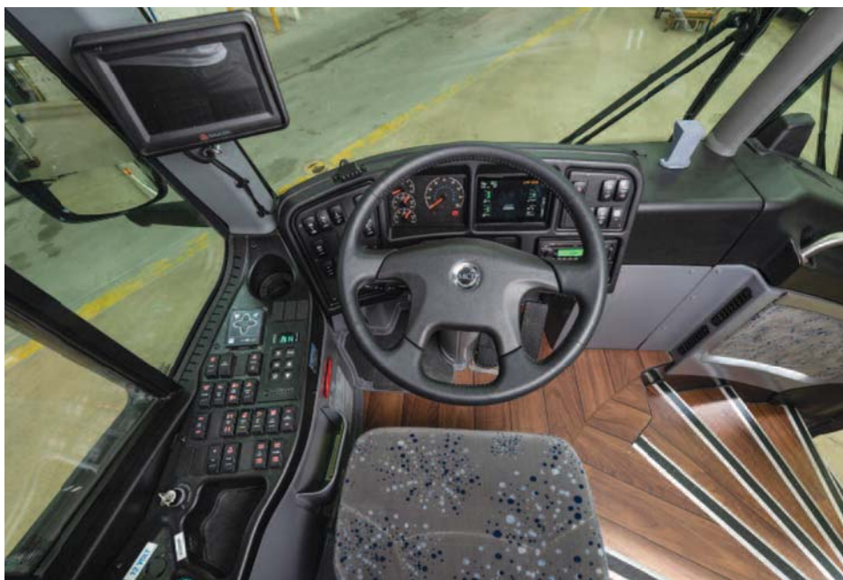
As with the other Next Generation "D" models, the D4520 incorporates the new design and technology introduced by the D45 CRT LE. Drivers will appreciate the narrower pillars that increase driver visibility. Other updates include a redesigned ergonomic dash and a lower instrument panel that provides better sight lines while putting intuitive controls within reach.
