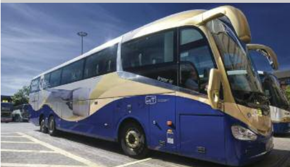
Translink is the provider of public transport in Northern Ireland. Metro and Glider Services operate in the Belfast area while Ulsterbus and Goldline bus services connect the rest of Northern Ireland. This Translink Goldline bus incorporates an Irizar i6 body with a Scania chassis. TRANSLINK.
