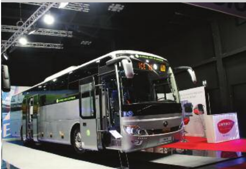
The Chinese have been leaders in developing and building electric buses and coaches. Shown here is a Yutong Ce12, an electric touring coach. It has two doors and a range of about 137 miles. The photo was taken at a recent Busworld event in Kortrijk, Belgium.
