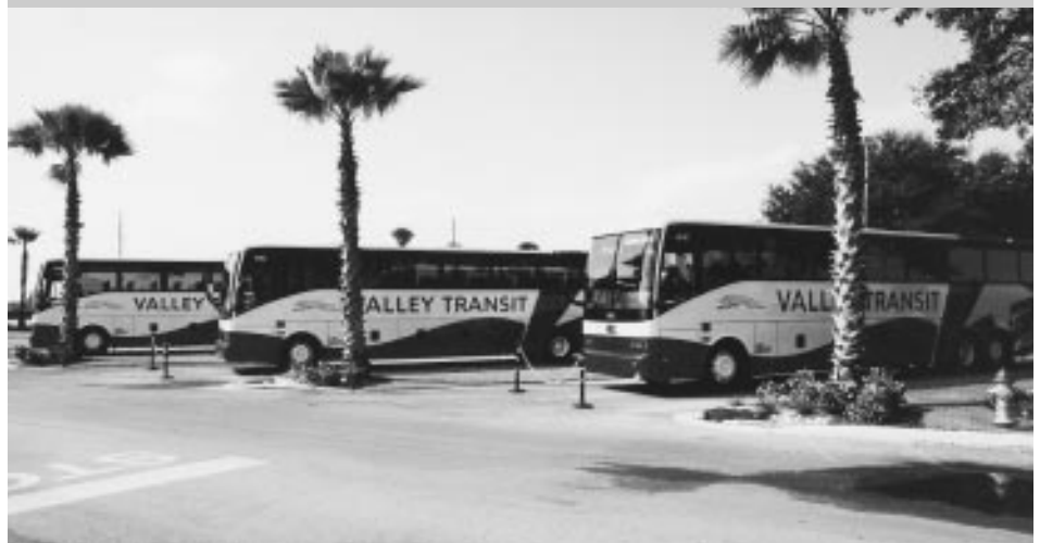
Three of the eight new Van Hool C2045 coaches were photographed at ABC Bus in Winter Garden, Florida, prior to delivery. The people from Valley Transit indicate that these coaches will be "the first coaches in South Texas with 57-passenger seating and theater quality digital audio/video entertainment systems." All of the coaches have a 370-horsepower Detroit Diesel engine, flush toilets and Amaya Gaudi seats. ABC BUS.
