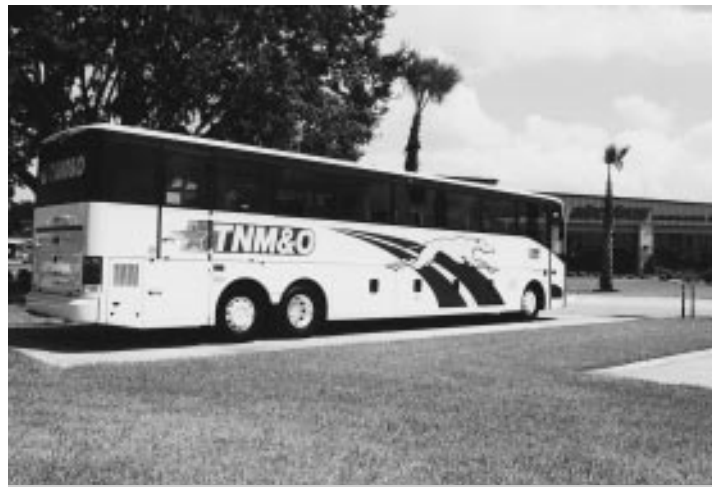
One of the 11 new Van Hool coaches for TNM&O was photographed at ABC Bus in Winter Garden, Florida, prior to delivery. If you look closely, you can see the door for the Steward & Stevenson lift behind the tag axle. Other features of the coach include an Isringhausen model 6800 driver's seat, a flush type toilet and a central locking system. ABC BUS.
