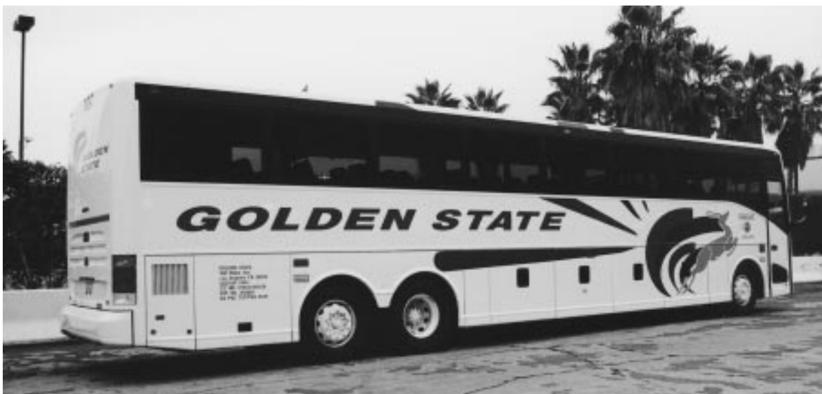
This C2045 was photographed shortly after delivery to Golden State Transportation Company which is based in Los Angeles, California. All of the 10 new C2045 coaches have Detroit Diesel engines and Allison automatic transmissions. Van Hool seating for 59 passengers is provided and special features include an REI four-monitor video system as well as a Monogram flush toilet. ABC BUS.
