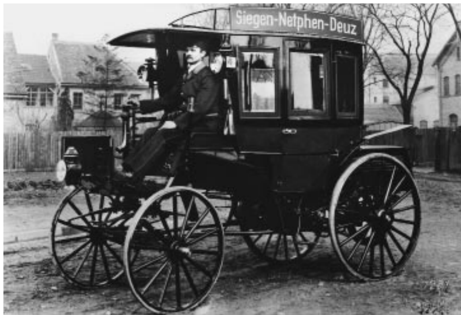
The connection between buses and stage coaches may not be as obvious today, but it was a century ago. Generally considered to be the first real bus, this vehicle started the first omnibus line in 1895 which ran between Wiegen, Netphen and Deuz in Germany. Its origin as a stage coach is obvious. Note the tiller instead of a steering wheel and the baggage area on the roof. MERCEDES-BENZ/NBT COLLECTION.
