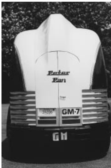
The Futurliners had a fairly plain back end. But in many respects they were similar to the first GM Silversides buses and were built on the bus assembly line in Pontiac, Michigan. This photo is of GM-7, the Futurliner restored by Peter Pan Bus Lines. PETER PAN.
