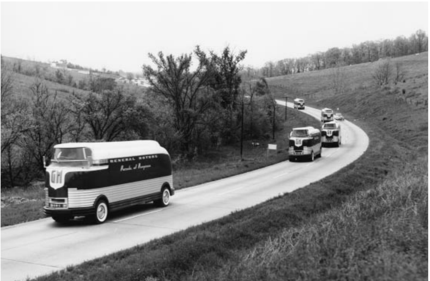
The Futurliner driver sat with his head 11 feet above the ground. That bubble cab was hot until these little roofs were put over it during the 1953 rebuilding. There were two jump seats behind the driver for additional staff if necessary. Futurliner drivers had a radio receiver, but only the leading and trailing unit could transmit. THE GM FUTURLINER RESTORATION PROJECT.
