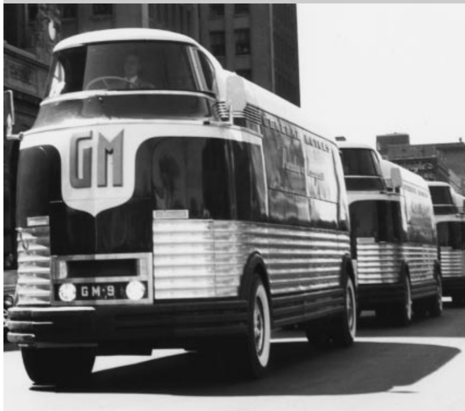
GM-9 leads a convoy of Futurliners during a ceremony in Detroit in May of 1952 to kick off the revamped postwar Parade of Progress. Note that the bubble driver's area has been roofed over to keep out the sun. THE GM FUTURLINER RESTORATION PROJECT.
