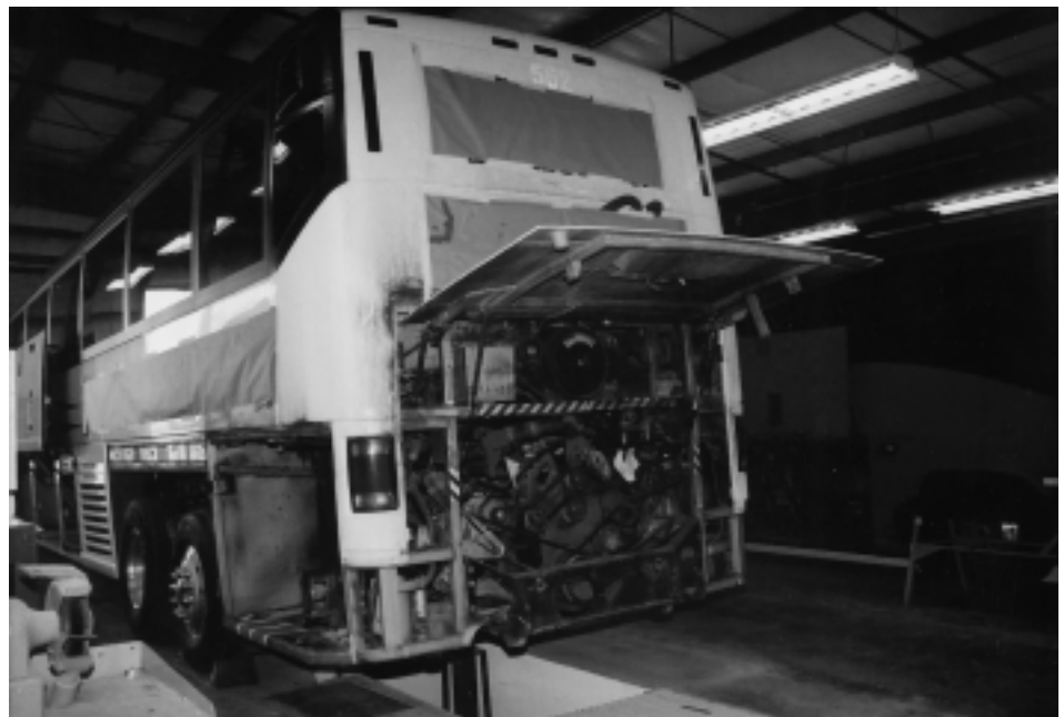
Although technically not a collision repair, some time was spent discussing engine compartment fires. There are several possible causes for engine compartment fires including turbo failures. Most are expensive to repair because of wire harness damage. NBT.
