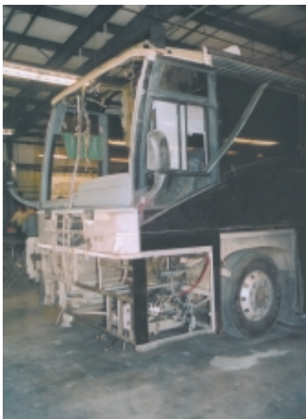
One of the buses in the collision repair shop suffered substantial front end damage. Attendees were able to view repair work in progress. In this case both major frame work as well as replacement of wiring harnesses was necessary. NBT.
