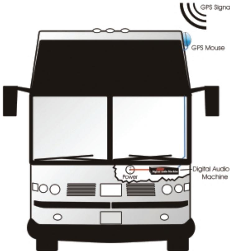
The Digital Audio Machine has no moving parts and takes advantage of state-of-the-art technology. A GPS mouse continually monitors the location of the vehicle and can be as accurate as five meters. When the Digital Audio Machine finds a match in its memory for the location, it automatically plays the associated pre-recorded announcements. ALCORN MCBRIDE.
