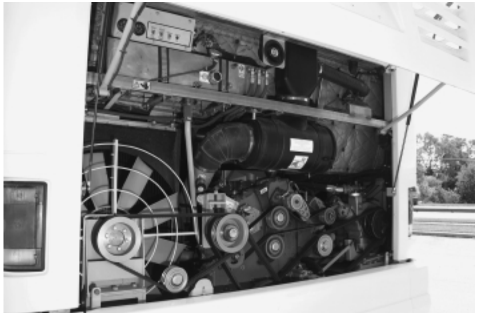
While the Series 60 engine is somewhat traditional, there are numerous changes and improvements in the engine compartment. Linnig clutches are used instead of a miter box on the fan. In addition, checking filters is greatly simplified with filter minder sensor gauges. The engine coolant filler is located at the top of the compartment - follow the overflow line up to the cap. MCI PHOTO BY JOHN MERKLE.
