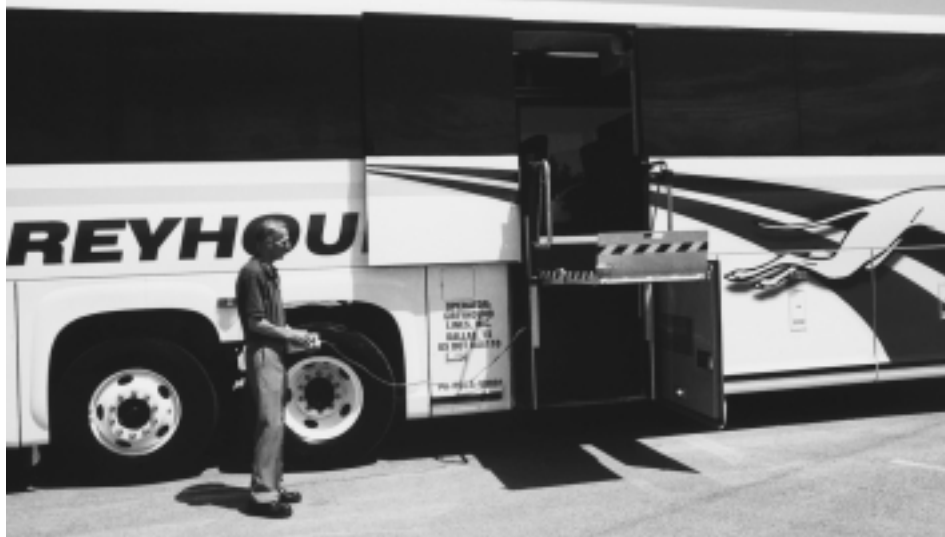
The G4500 comes with a Stewart and Stevenson bay lift and is installed similar to the lifts on the E4500 and J4500 models. However, a sliding door is used similar to that found on the D4500. Passenger seats are mounted on tracks and are easily moved. Belts for securing the wheelchair are mounted to the seat frames and are easy to use. NBT.
