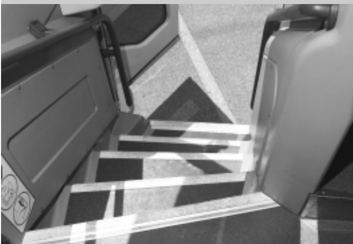
The passenger entryway on the G4500 is tapered but does not curve as much as on the E4500. The door is held at three locations to provide a good seal, and the door itself has more glass with a larger lower window.
