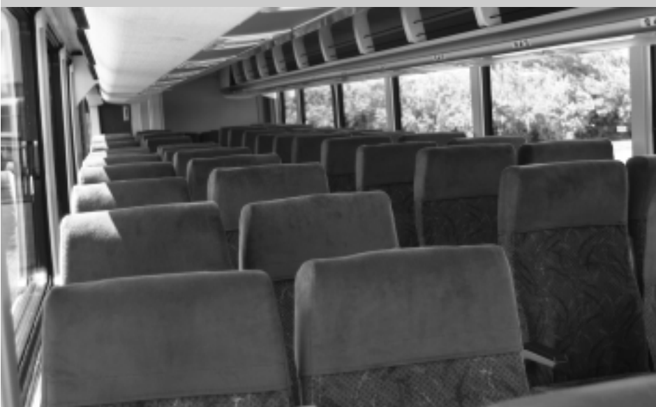
Greyhound has open luggage compartments and Amaya seats which give the interior a typical line haul appearance, albeit more modern than previous models. However, options are available for other seats, enclosed parcel racks, a video system and other amenities to turn the coach into a stylish tour vehicle. MCI PHOTO BY JOHN MERKLE.
