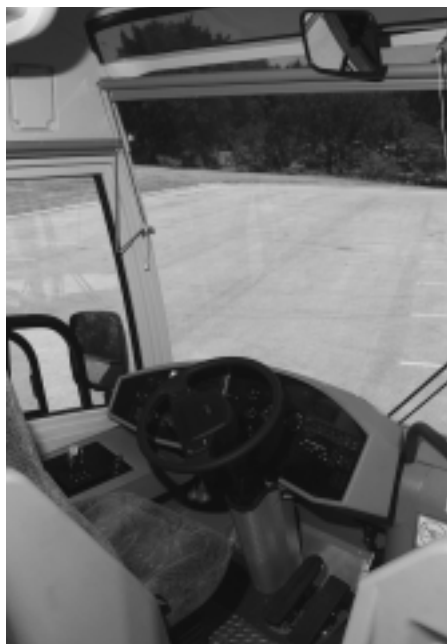
The driver's area is open and offers a good view of the road. In the center of the dash is a multiplexed section with lights and gauges while rocker switches are used on the side panels. Transmission and parking brake buttons are on the left. MCI PHOTO BY JOHN MERKLE.
