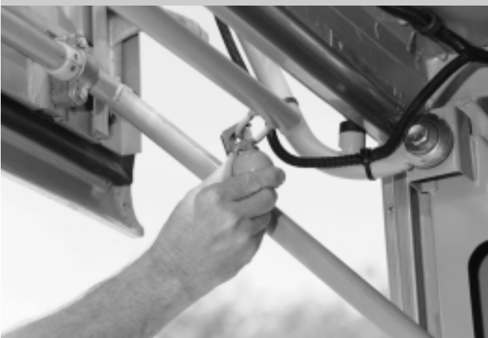
Mechanical arms replace gas cylinders on compartment doors to reduce maintenance costs. This little yellow knob locks the compartment door in the open position to prevent its closing on luggage or a driver's hand.
