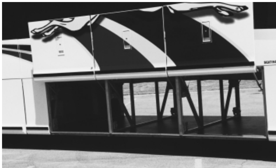
If you look carefully just below the windows, you can see the dimple or bow in the side of the coach which aerodynamically channels road grease and dirt away from the passenger windows. The underfloor luggage compartment is much more open than previous MCI models and offers an impressive 440 cubic feet of storage space. NBT.
