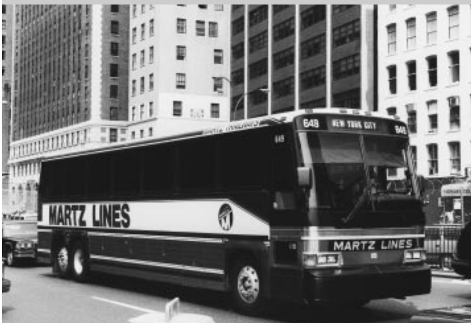
The "B" models replaced the "A" models after the 102C3 was already in production. Both a 96-inch and a 102-inch wide version of the "B" were offered. This 96B3 was operated by Frank Martz Coach Lines and was photographed in New York City in 1995. J.C. REBIS JR.
