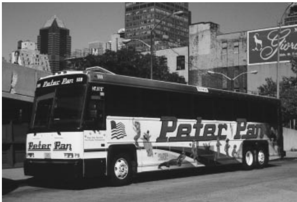
Originally developed as a handicapped-accessible coach in 1988, the 45-foot 102DL3 went into regular production in late 1992 and soon became MCI's most popular model – a distinction it still retains. In addition to the 45-foot length, the 102DL3 offered the new Series 60 engine and a steerable tag axle to decrease turning radius. This example of the 102DL3 is operated by Peter Pan Bus Lines and was photographed in New York City in August of 1998. J.C. REBIS JR.
