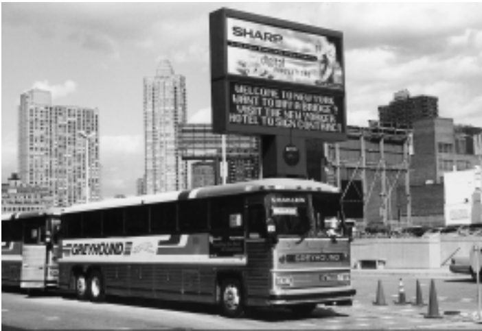
Built from 1992 through 1999, the MC-12 model became the backbone of the Greyhound fleet in the late 1990s. With a width of 96 inches and a length of 40 feet, the MC-12 was more of a refinement of an existing design than a new development. This 1992 MC-12 was photographed at the Jacob K. Javits Convention Center in New York City on April 10, 2000. J.C. REBIS JR.
