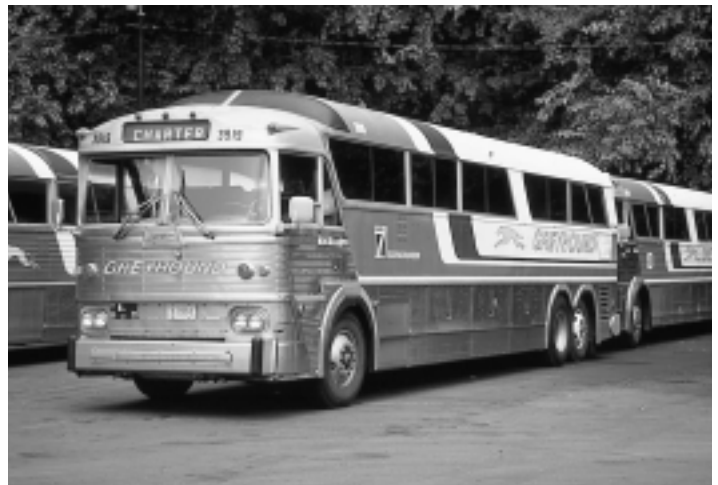
The MC-7 went into production in 1968 and became MCI's first 40-foot coach. It effectively replaced the Scenicruisers in Greyhound's fleet and became popular with other operators. This example, with the "Super 7 Scenicruiser" logo, was photographed in Harrisburg, Pennsylvania in September of 1979. ROBERT REDDEN, REDDEN ARCHIVES.
