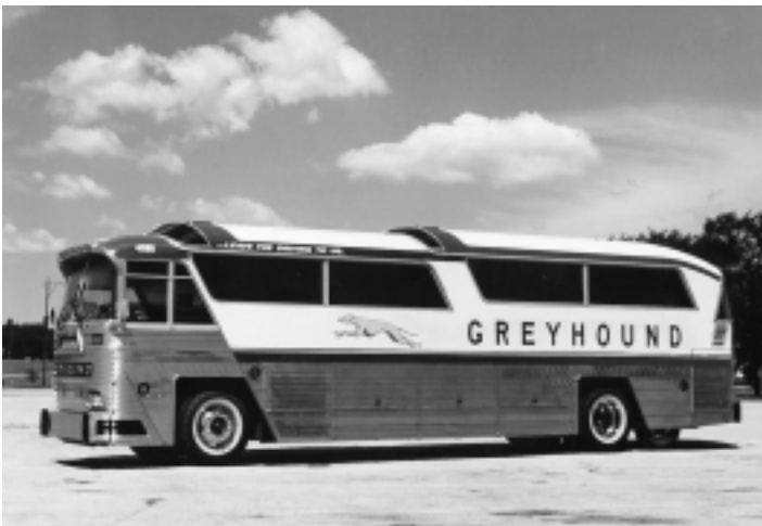
Several people suggest that the MC-6 was originally intended to be a replacement for the aging Scenicruisers. It has an unusual design and pioneered the new 102-inch coach. When acceptance of the new width was not forthcoming, only 100 were built. They operated on special routes with permits. NBT.
