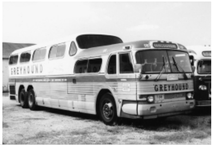
Greyhound's PD4501 Scenicruiser represented a major step forward in bus development. Left: The GX-2 prototype of 1949 was responsible for obtaining approval for 40-foot coaches on American highways. It also pioneered several new systems and developments. Right: The PD4501 Scenicruiser, an exclusive model for Greyhound, entered regular production in 1954. It not only was the first production run of 40-foot coaches but also represented the first model where air conditioning and a restroom were standard equipment. This one was photographed in Oklahoma City in 1972. FRED RAYMAN.
