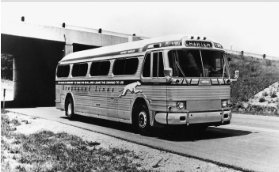
The PD4104 introduced air ride suspension and offered both power steering and a restroom. Greyhound became the largest buyer and operator of the PD4104 although it was also available to other bus companies. Greyhound's pre-Scenicruiser PD4104 coaches built in 1953 and 1954 were delivered without restrooms. Those delivered after the Scenicruisers from 1957 to 1960 came with restrooms and an improved air conditioning system. NBT.
