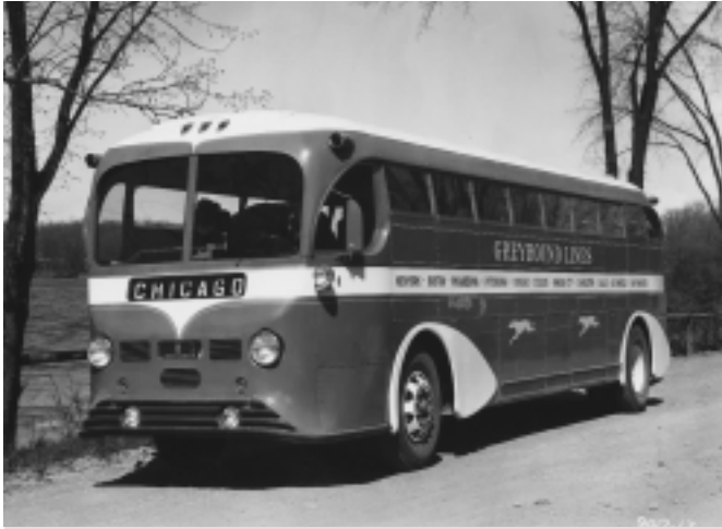
Built in 1935, the X-1 was one of three pilot models for the new 719 developed by Dwight Austin and Yellow Coach. It revolutionized intercity bus design with its flat front, enclosed underfloor luggage compartments and rear engine.
