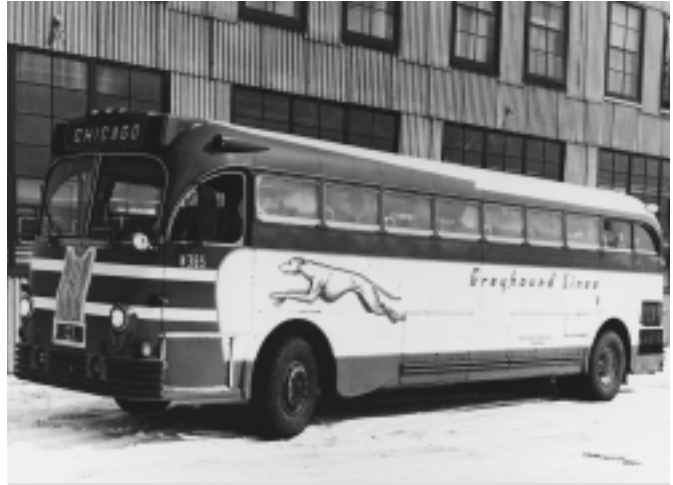
Introduced in 1936, the Yellow Coach model 719 "Super Coach" became the new flagship model of the Greyhound fleet and revolutionized the intercity bus industry. The following model 743 introduced air conditioning and the diesel engine.
