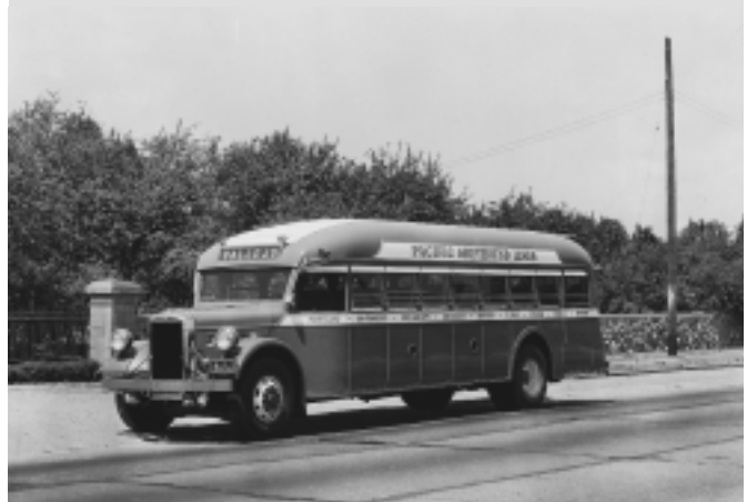
This 1934 Yellow coach model 788 showed an early attempt at streamlining with rounded corners. An extended roof rack for luggage was added later.
