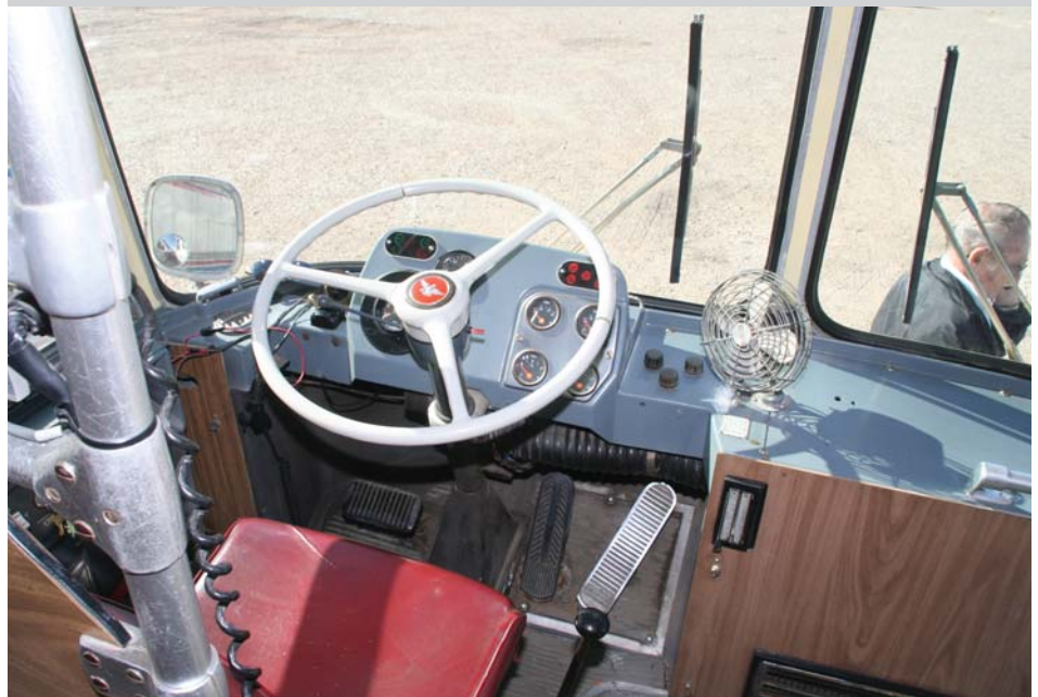
This recent photo of the Eagle shows that the driver's cockpit area has been substantially restored including the dash and the Eagle insignia in the middle of the steering wheel. The coach retains its manual transmission and clutch. However, the original engine was replaced by one found in NATIONAL BUS TRADER. NBT.
