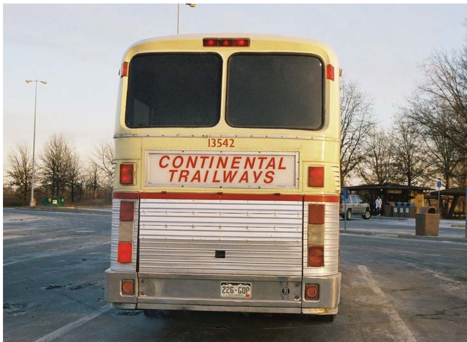
Larry Yohe took great pains to restore the coach to its original appearance. The illuminated sign box on the rear, below the rear windows and above the engine compartment doors, came from another Eagle. The actual sign itself had to be painted and recreated from scratch. LARRY YOHE.
