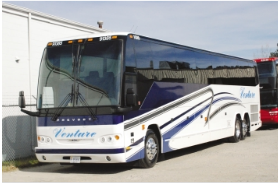
This 2009 Prevost H3-45 was originally delivered with a standard seating capacity of 56 passengers. In November of 2008, it was outfitted with 30 wide leather seats with six regular seats remaining in the rear. From November to March, the coach will be configured to seat 36 passengers for sports teams. From April to October, the coach will be used with a 56-passenger configuration for the busy charter season.
