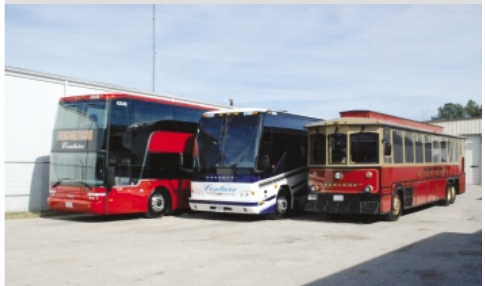
Three different buses in the current fleet, from left to right: One of the two new Van Hool TD925 double-deck coaches. A 2009 Prevost with the Volvo engine and Allison transmission with a special interior for transporting sports teams. One of the two MC-8 coaches modified with a trolley appearance.
