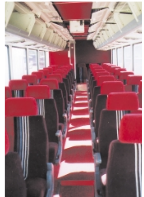
Shown here is the interior of one of the special 1990 102C3 coaches. With only 43 seats, these coaches offered additional legroom as well as a carpeted floor and enclosed parcel racks making a plush interior.
