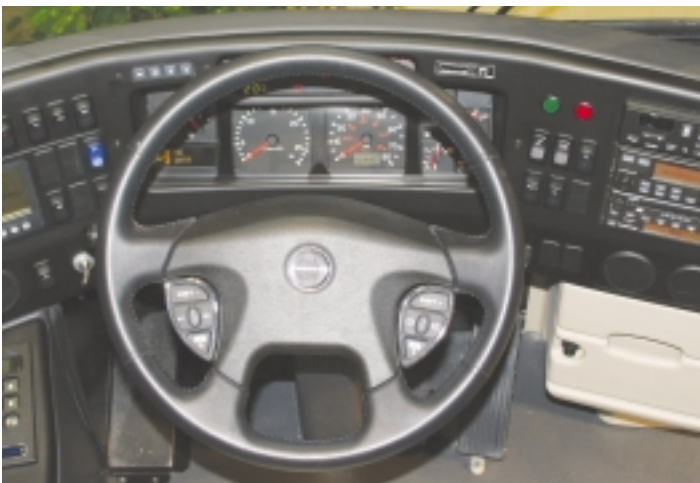
Prevost's new steering wheel now incorporates buttons for the cruise control, shifting, engine brake, horn and electric sun visor. Groups of buttons are located on each side of the wheel just below the center.
