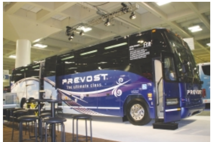
This new H3-45 was one of four different new coaches on display in the Prevost booth area. It is powered by the new Volvo D13 engine and has a wheelchair lift just forward of the rear wheels.
