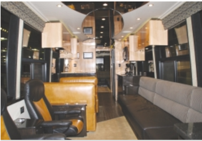
Located in the Prevost area was this H3-45 converted by Amadas Coach with an executive interior. A mid-galley and restroom floor plan allows seating for 24 passengers with a couch, dinette and chairs at the front and a U-shaped lounge at the rear.
