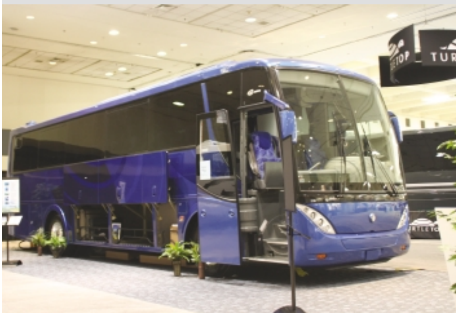
An interesting new exhibitor at this UMA Expo is Caio North America. They showed their G3400 model built by Caio Induscar in Brazil. With a length of 36 feet and seven inches, it provides seating for 38 passengers plus a restroom.
