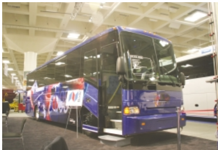
Built on a Freightliner chassis, ABC's new 3035RE offers big coach styling and features an economical 35-foot body-on-chassis bus. It is built in Michigan by Thor Industries for ABC and is at the top of its class in quality and amenities.
