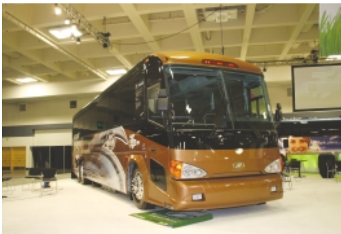
Recently updated, MCI's D4005 offers an interesting combination of tried-and-true technology with a modernized appearance. With a length of 40 feet, the coach seats 43 passengers and is ideal for mid-size groups.
