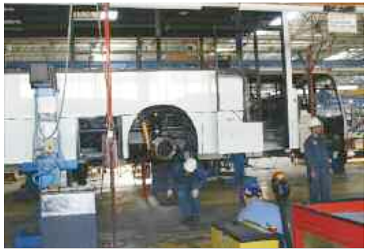
Temsa uses multiple bus assembly lines with similar models assigned to the same line. Several supplier companies are also on the premises to provide a range of components and services ranging from painting to seats and tires.
