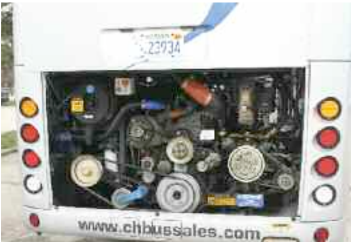
Shown here is the engine compartment of a TS-30. Both models offer a reliable power train consisting of a Cummins engine and an Allison transmission.
