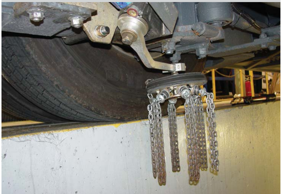
Also optionally available are Automatic Tire Chains. Attached to a disk and mounted on the rear axle, the chains spin and pass under the drive tires when in operation. This provides welcome traction on ice and snow.
