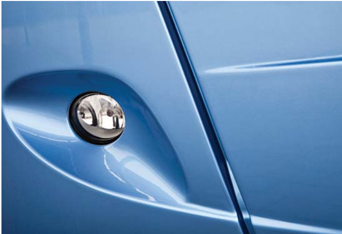
The Setra cornering lights are combined with the fog light system. They come on automatically when turning to give the driver some welcome illumination as the coach comes around a corner.
