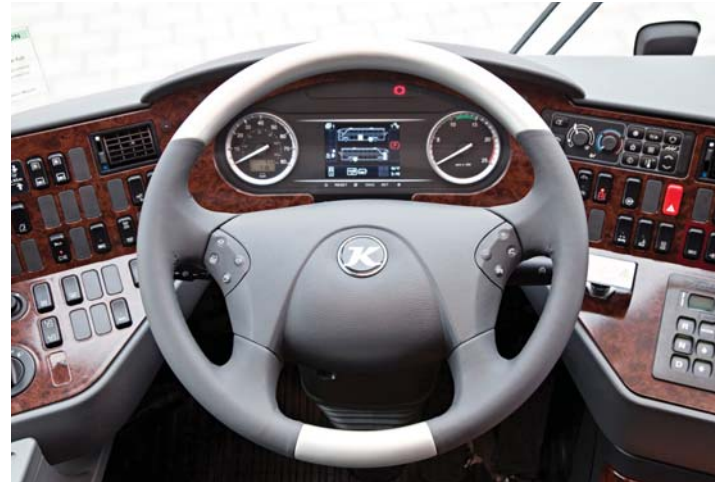
Drivers of the Setra S 417 will now find audio and video controls mounted on the steering wheel. This arrangement improves safety by eliminating the need for the driver to stretch and reach while driving.
