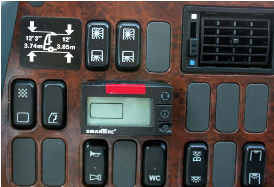
Optionally available from Setra is the Tire Pressure Monitoring System. A display on the dash eliminates the need for taking tire pressures with a gauge and hence makes monitoring tires much easier for your drivers.
