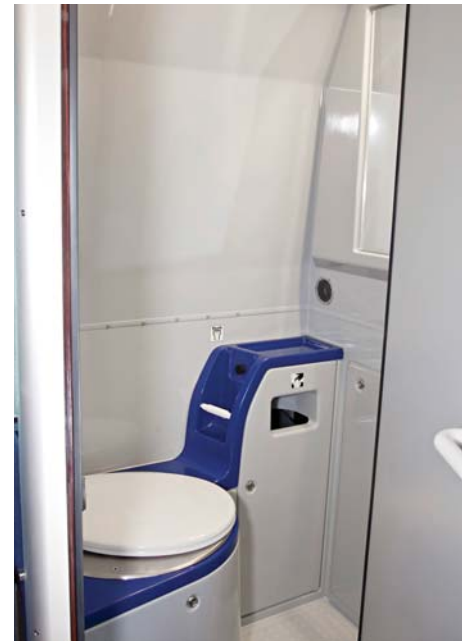
The rear-facing lavatory reduces the risk of injury in the event of a braking situation or emergency deceleration.
