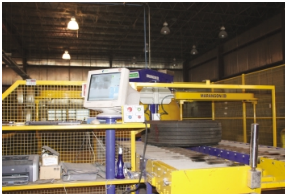
The Shearography machine uses state-of-the-art technology to check incoming tires for possible problems. It takes photos of the tire both with and without a vacuum and compares them using computer technology to look for problems. The tire shown came from Peoria Charter Coach for retreading.
