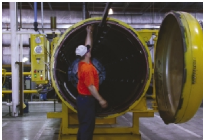
Brahler's uses a steam autoclave to cure the retreaded tires. Not only does the steam prevent the tire from drying out during curing, but it also holds the length of the curing process to only 94 minutes. BRAHLER'S.
