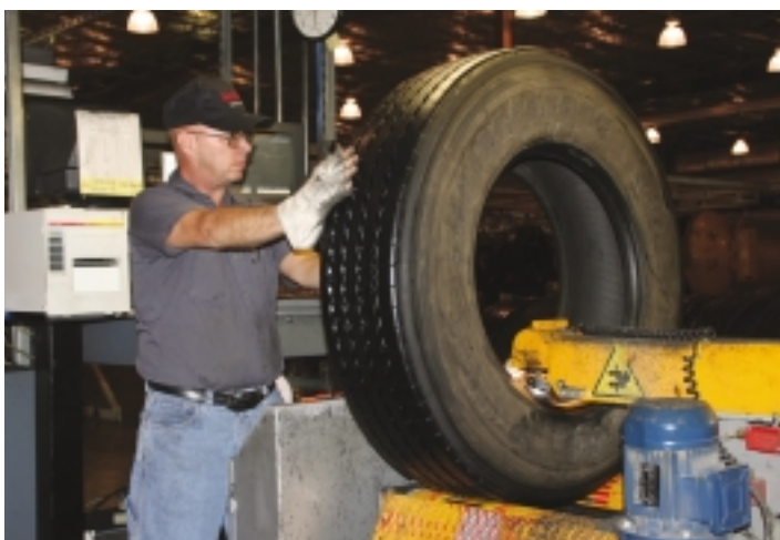
After being cured, the retreaded tires are cooled at room temperature and then go through a final inspection. The inspector has full authority to reject tires or send them back to any station.
