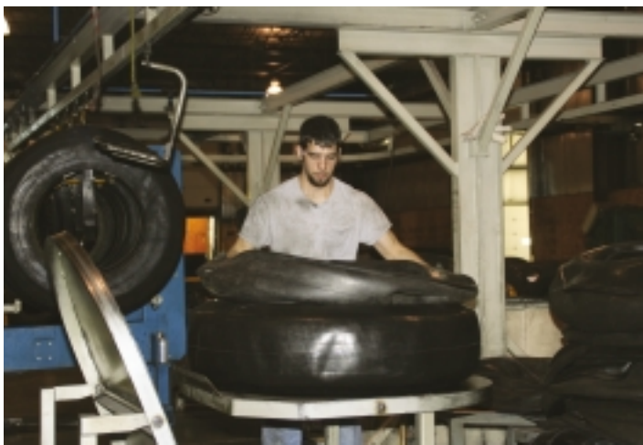
Station nine takes the tire with its new tread and puts it into a rubber sleeve called an envelope. In this photo, the outer envelope has already been placed and the technician is inserting an inner envelope.
