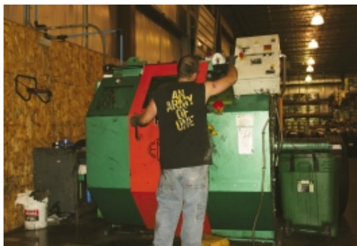
Tires at Brahler's also go through an actual pressure testing where they are placed in a cabinet to protect the technician while they are subjected to increasing pressures as a final test.
