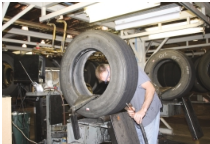
Tires with problems discovered in the Skiving process are sent to the Repair Station where any hole is repaired using a TECH thermocure patch that is stronger than the original line.
