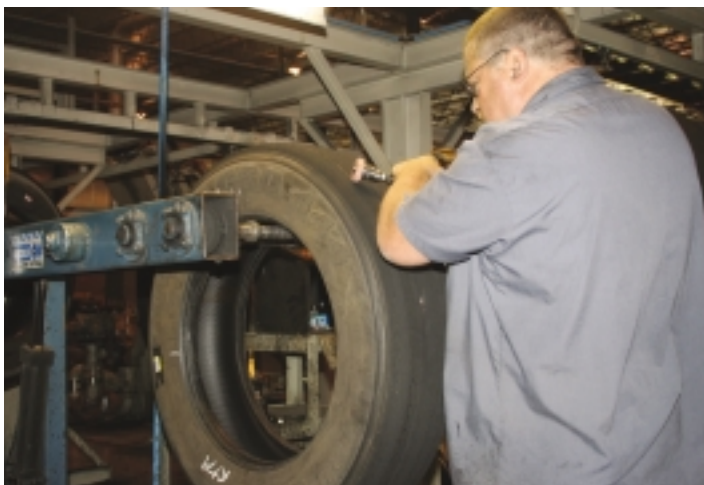
Once the excess rubber tread is removed, the tire goes through yet another inspection where trained technicians probe for tire holes or defects in a process known as Skiving.
