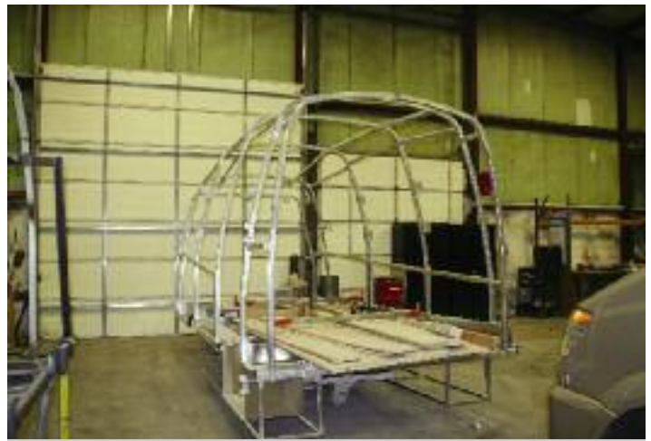
Like the big coaches, the carlines and body frame of the Mauck2 are made from tubular steel. Galvanized steel is used for increased longevity over mild carbon steel.
