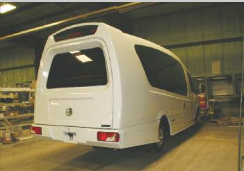
This Mauck2 towards the end of the assembly line shows some of the new improvements. The body was remoulded to utilize new taillights and cab marker lights that are easier to source and work better with the Sprinter wiring harness. This unit also has the new three-panel windows.
