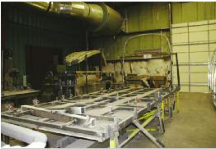
Increased sales at Mauck2 has prompted a move to more sophisticated manufacturing operations. Like the big coaches, production now begins with this frame welding jig.
