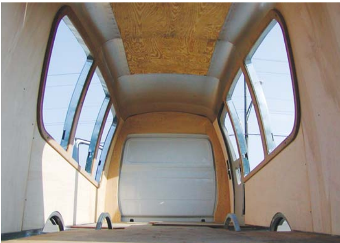
A major advantage of the Mauck2 body is that it offers 10 more inches of space between the walls at the floor level than the standard Sprinter body. This provides considerably more space for interior customization.
