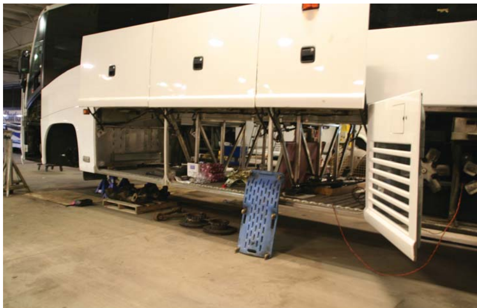
MCI uses a 210+ point inspection on coaches going into the Select+ or Certified++ levels of the pre-owned coach program. Taken at the MCI facility in Des Plaines, Illinois, this coach was being torn down for inspection. Note that in addition to checking systems and components, the wheels have been removed for inspection.
