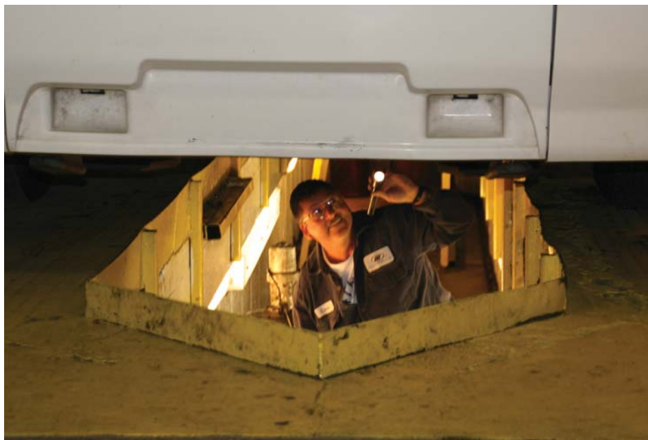
The MCI inspection for the pre-owned coach program covers virtually every corner of the coach. Included is a thorough inspection of the running gear, suspension system and steering system. Here, Oscar Chacon, a technician at the MCI Service Center in Des Plaines, Illinois, is down in a pit doing a thorough inspection of a coach going into MCI's new pre-owned coach program.
