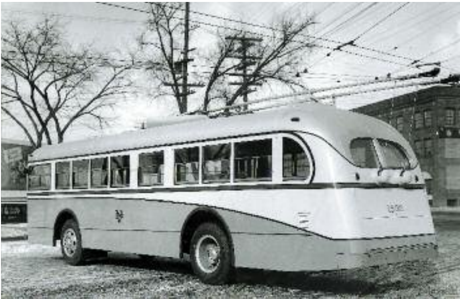
In spite of the war effort, MCI did build a bus in 1942. It was a city transit bus powered by overhead trolley wires and was reportedly the first trolley bus built in Canada. It operated in Winnipeg for 25 years.
