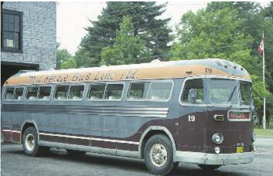
MCI's Model 96 was the last major model prior to the start of the MC-1 series. It was introduced in 1956 and was built into 1960, even after the MC-1 was introduced. This example was operated by Mac Kenzie Bus Line Ltd.
