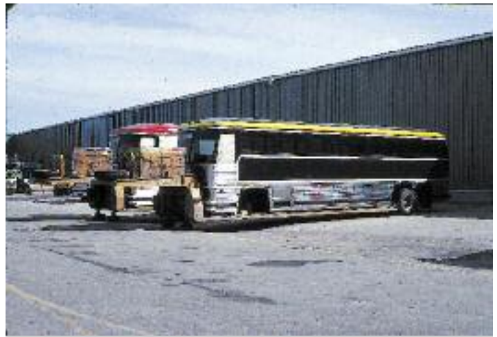
With the opening of the new Fort Garry facility, new coaches were partially completed up there. Then, the shells were transported on flatbed trucks across the border to Pembina where they were completed.
