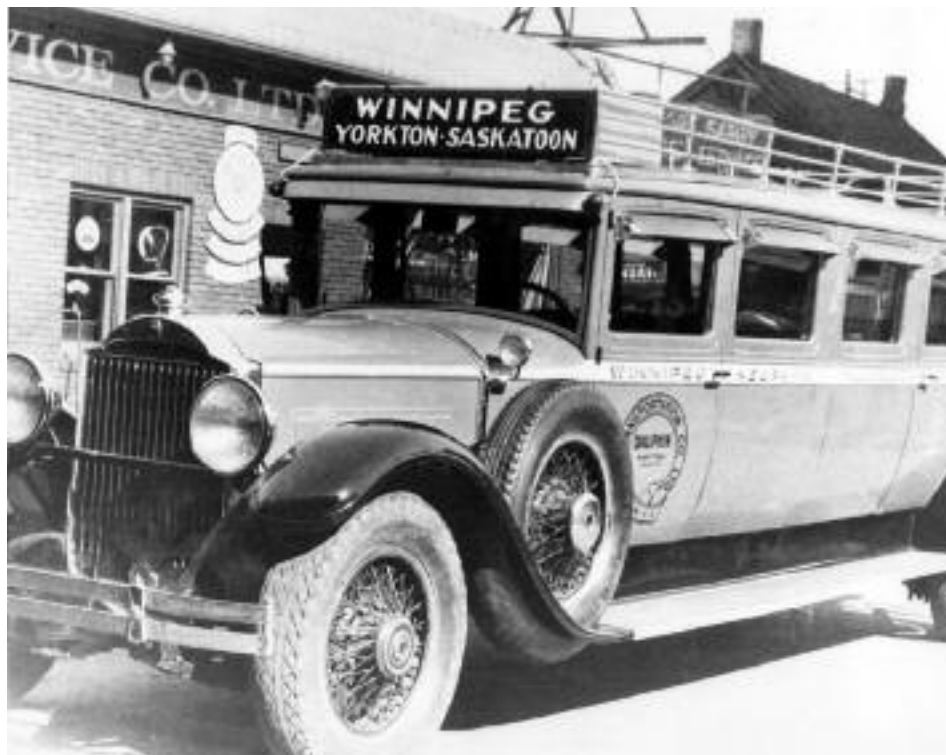
The Fort Garry Motor Body and Paint Works built their first bus in 1933. It consisted of a stretched 11-passenger body on a Packard car chassis. In following years the company built larger bodies and put them on truck chassis.
