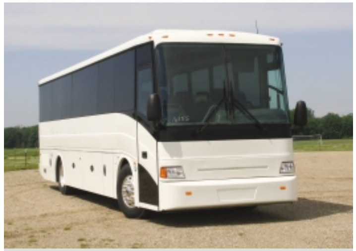
The 3035RE from ABC Companies is built by GCA. It uses an FCCC XB-R raised rail chassis and offers numerous big coach features including a restroom and underfloor luggage compartments. NBT.
