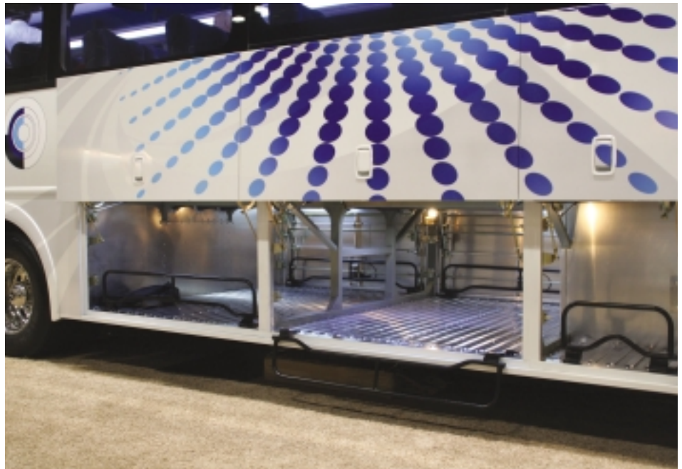
The versatility of the FCCC staff and products can be seen in the XB-R chassis used on the Caio bus. Upper C-channels on the XB-R chassis are effectively replaced by the body super-structure on the Caio G3400. This provides several advantages including increased baggage capacity. The folks from Caio were so impressed with their baggage capacity that they showed it off at the UMA Motorcoach Expo in Orlando in January of 2009. NBT.
