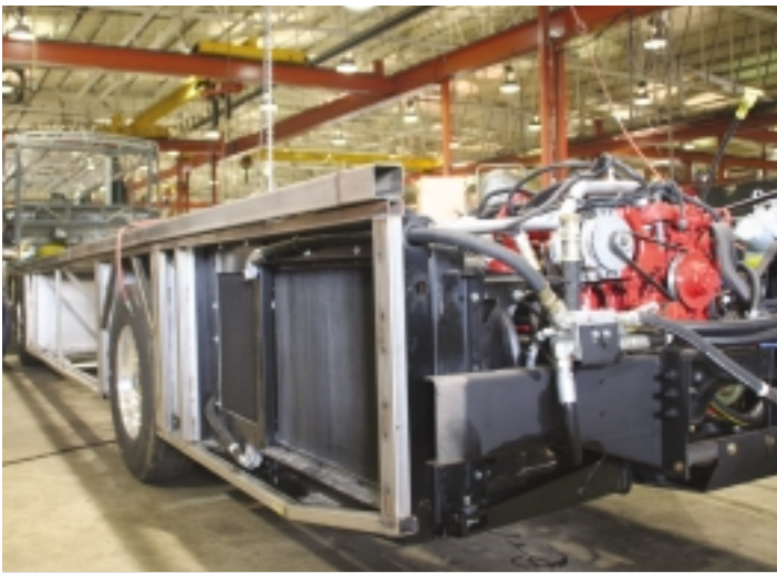
The FCCC XB-R chassis is shown at the start of the General Coach America assembly line at their plant in Imlay City, Michigan. CGA builds the 3035RE bus for ABC Companies. NBT.
