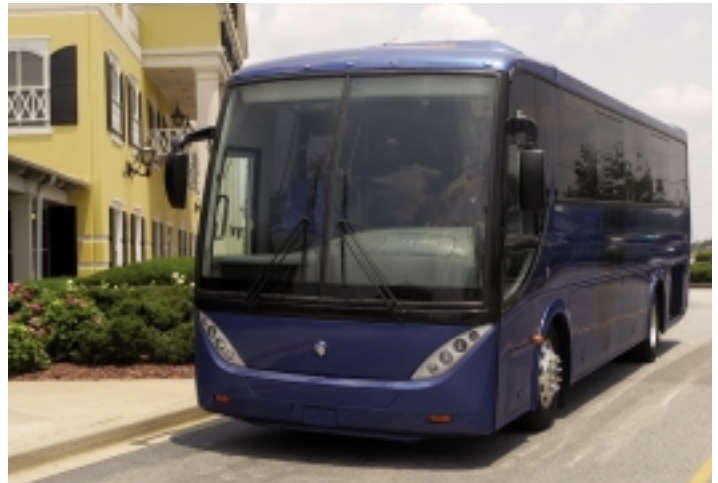
The Caio G3400 mates a body from Brazil with an XB-R chassis. What results is a mid-size rear-engine bus with a big coach appearance and numerous big coach features. FCCC.
