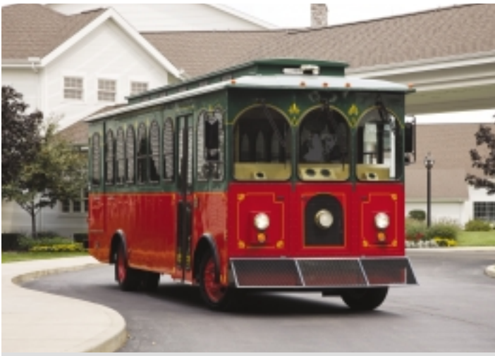
The Supreme Trolley is built on an FCCC MB-55 chassis and is sold by Specialty Vehicles. The MB-55 chassis is popular for various specialized applications including trolley-themed buses. FCCC.
