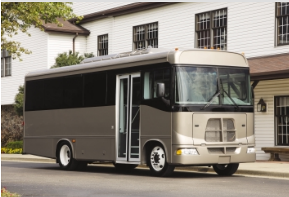
Among the upscale mid-size buses offered in recent years is the Apollo from Glaval Bus Corp. Built on a FCCC MB-55 chassis, the Apollo offers a significant step up from the traditional cutaway styling. FCCC.
