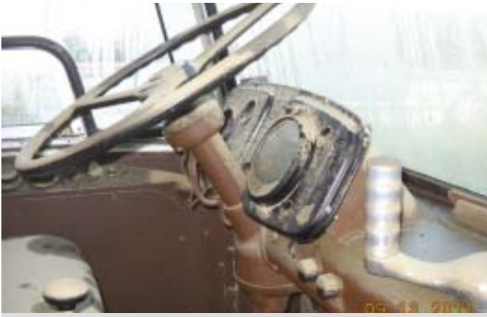
Taken on or about Tuesday, September 13, this photo shows the steering wheel and dash of the Capitol PD4106. While nothing is obviously broken, a film of brown mud covered most surfaces. JOT BENNETT.
