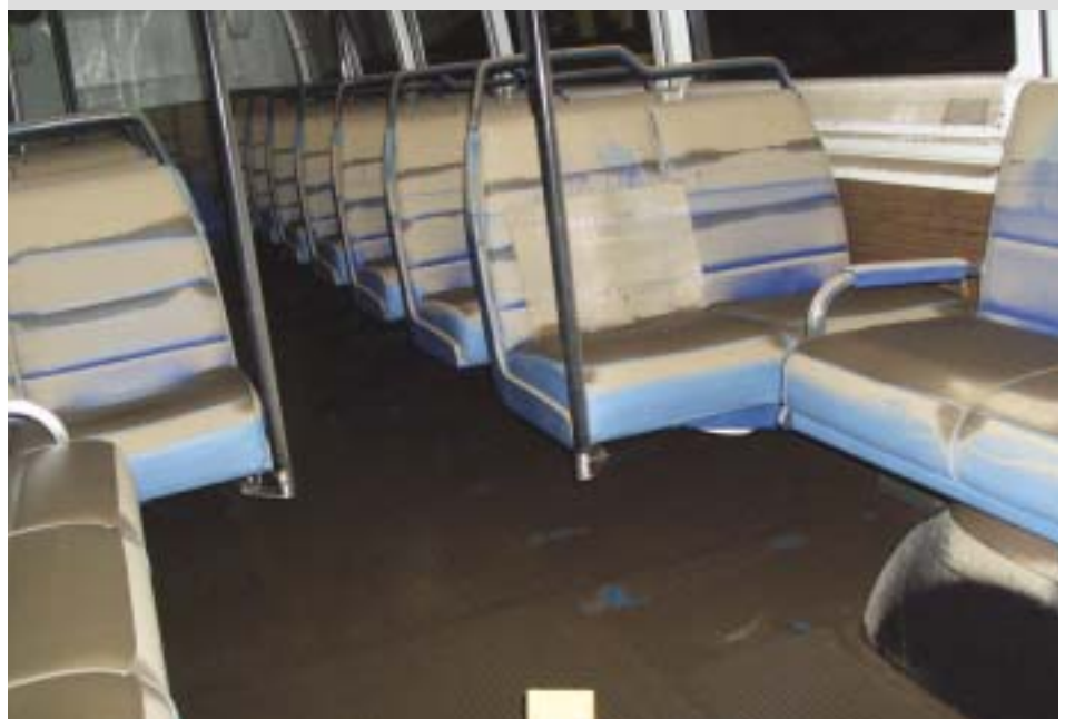
This photo shows the interior of one of the transit buses, probably the RTS. A brown film of mud covers many surfaces. A restoration firm was somewhat hopeful and said that they had seen and worked with worse. THOMAS MOZER.
