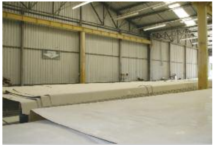
CAIO builds its own roofs in one piece to eliminate seams and leaks. There also is an in-house glass operation.
