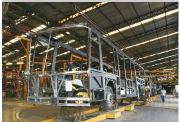
At this point on the assembly line CAIO buses are turned on a turntable and sent down the next line. Note the quality web frame construction.
