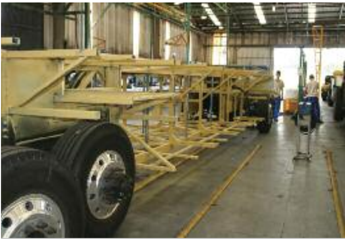
This integral bus on the CAIO assembly line shows its web frame structure between components rather than chassis rails.
