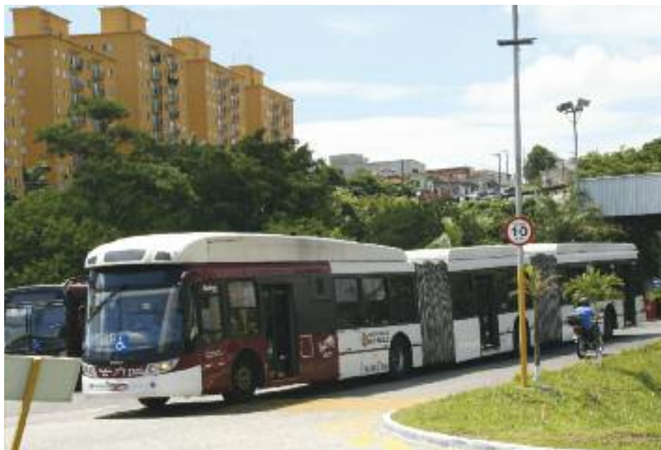
Public transit in Sao Paulo heavily depends on diesel buses. Shown here is a CAIO three-section Bus Rapid Transit (BRT) articulated bus. Note the additional doors on this side so these buses can operate in dedicated center lanes and stop at loading areas in the center of the streets.
