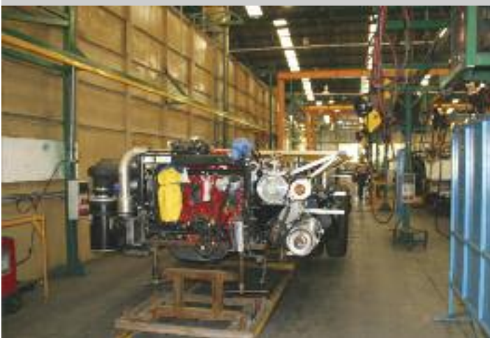
CAIO rolls their buses down the assembly line on these wheeled rail carts to eliminate any torsion or quality problems with tires on the floor.
