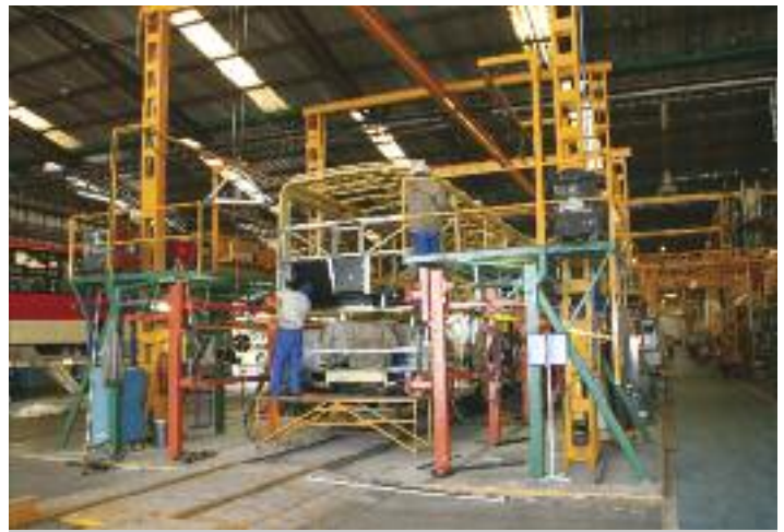
Jigs and other guides ensure a high-quality web frame on CAIO coaches. This one is being moved on one of the little rail carts.
