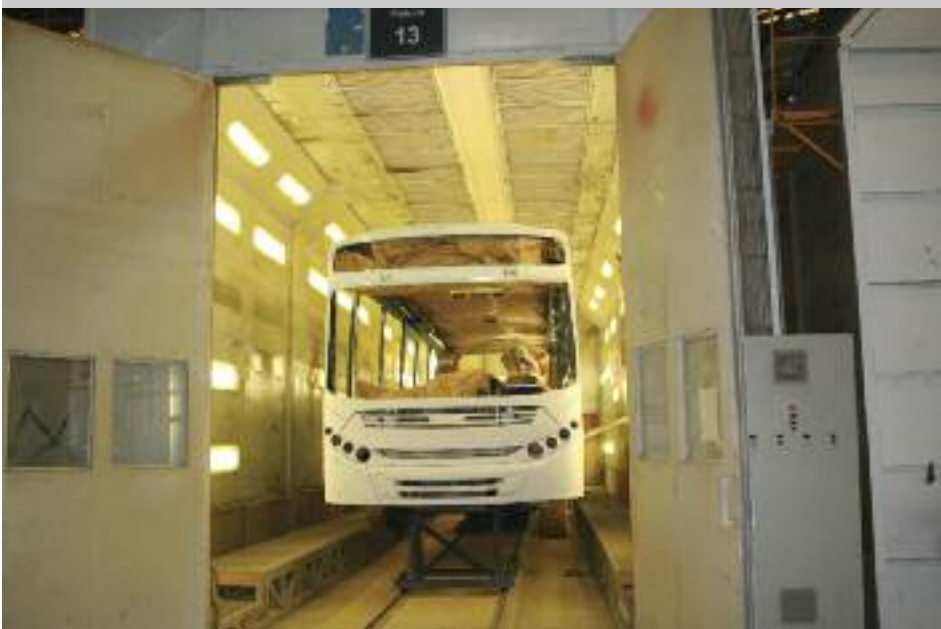
Still on its little wheeled cart, this CAIO bus is going through one of many paint booths. As is typical with higher quality coaches, the buses receive both primer and final painting. This area of the factory is due for some updating in the near future.
