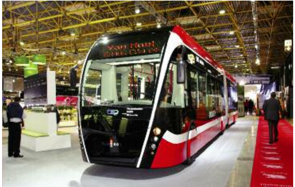
Van Hool's new Exqui.city transit bus design offers Bus Rapid Transit capabilities with a new exterior designed to look like a tram. It is available as either a two- or three-section articulated with hybrid, fuel cell or trolley bus power. Van Hool has already received three orders. This bus on display was a trolley bus with two poles at the rear.
