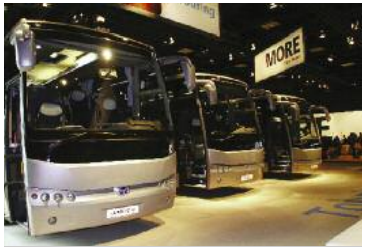
On the left, the new Tamsa Safari HD 14 is the newest addition to the Safari product line. It is a high-deck model with a length of 14 meters and is built with stainless steel.
