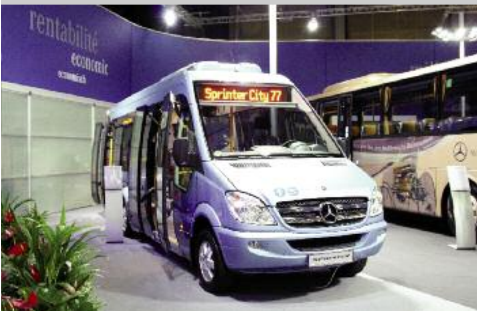
The new Sprinter City 77 model opened several eyes. With three axles, two doors and a length of more than 28 feet, it can carry more than 40 passengers. Whether this or a similar model will become available in the United States remains to be seen.
