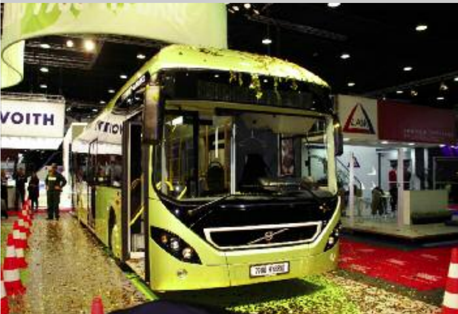
The gold foil on the bus and surrounding floor means that this photo was taken only moments after Volvo unveiled their new 7900 hybrid city bus. Replacing their 7700 model, the 7900 is similar in construction to Volvo's 8900 and offers a composite body and lighter weight. It is available with conventional diesel power, alternative fuels and hybrid power.
