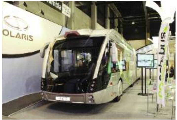
Solaris is a relatively new family-owned company located in Poland. They showed this Solaris Urbino articulated hybrid coach with BRT features and tram styling. It was built for a French operation.
