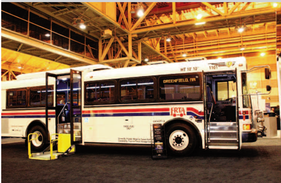
IC Bus showed their RE Commercial bus. It has a flat front design and is powered by a Maxxforce engine. This bus on display had a wheelchair lift at the back door.
