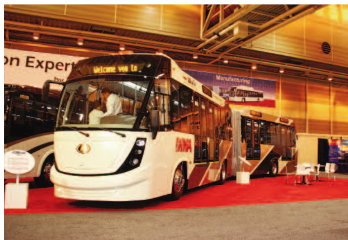
Dina's BRT articulated bus had platform doors on its left side for loading at high level platforms. Drivers would need some skill to bring the bus close to the platform without hitting it.
