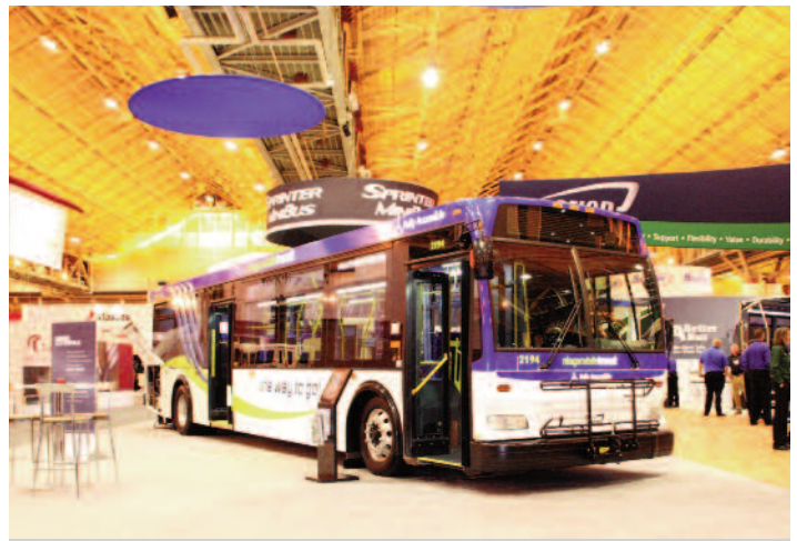
Sharing booth space with the Sprinter was this Orion VII low-floor Clean Diesel bus with a Cummins engine and a ramp for handicapped access.
