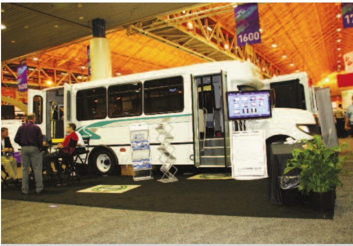
Champion Bus showed their UC Defender model. This mid-size cutaway was built on an IC Bus chassis and had a wheelchair lift at the curb at the rear.
