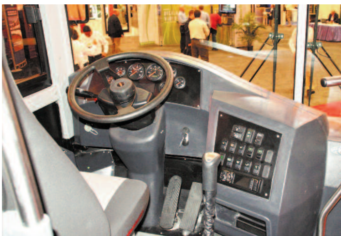
Dina's Linner model was essentially a short, suburban model with a rear door but no restroom. This photo shows the driver's area with the manual 6-speed Fuller transmission shift lever.
