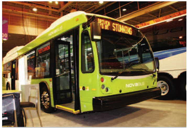
NovaBus showed their two-door hybrid electric transit bus. It had a Cummins 280 horsepower engine, a length of 40 feet and a seated capacity of 41 passengers.
