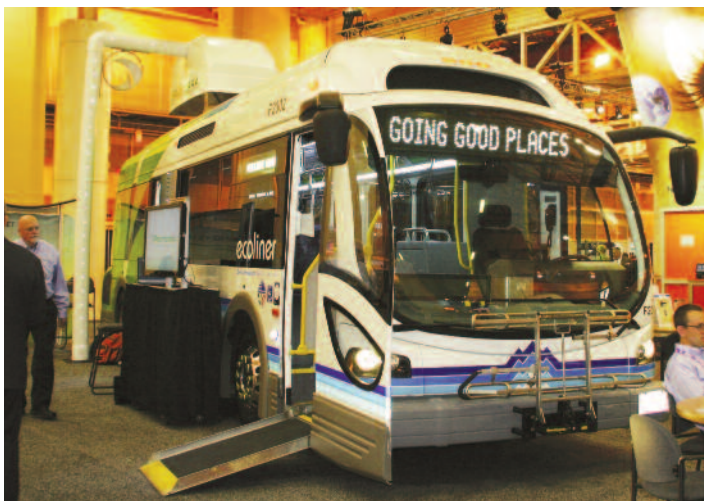
The Proterra battery-powered bus is already in service in Pomona. It uses an overhead charging station that recharges the bus in only 10 minutes.
