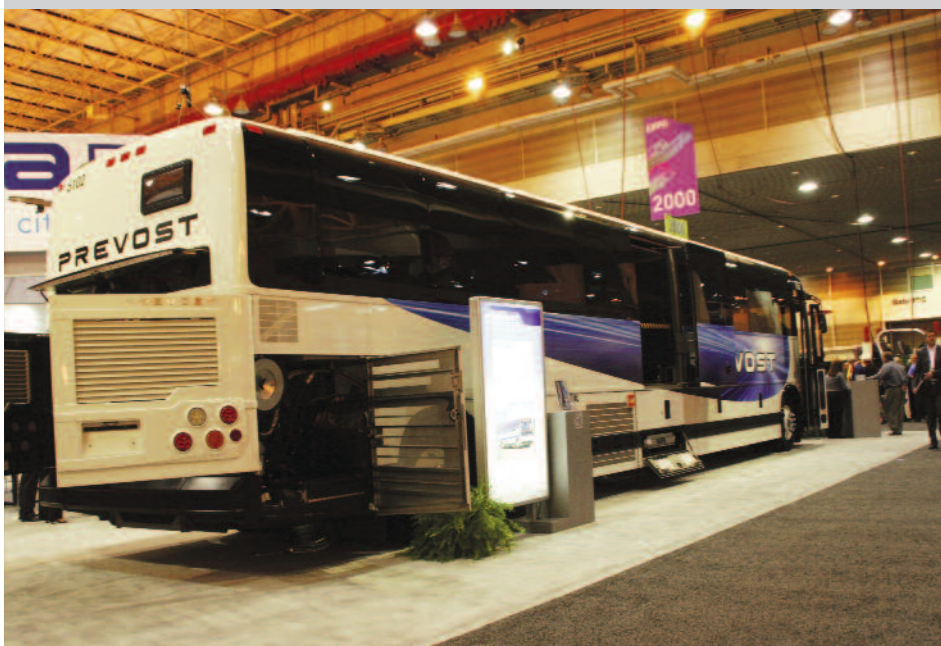
This Prevost Commuter Coach shared a booth area with two transit buses from NovaBus. This view looks towards the main walkway and shows the wheelchair lift and door towards the center of the coach. MTA in New York recently placed an initial order for 90 Prevost Commuter Coaches.
