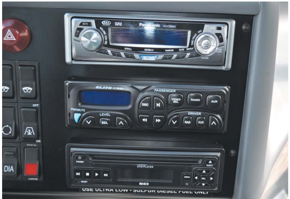
The refurbishing process includes both modernized and enhanced entertainment systems as well as an updated dash appearance. Note the installation of a new DVD player.
