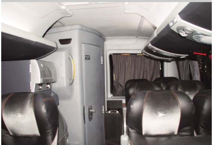
Marcopolo's Volare WL model is geared for higher quality travel with black leather seats, a restroom, a small galley area ahead of the restroom and a rear window.
