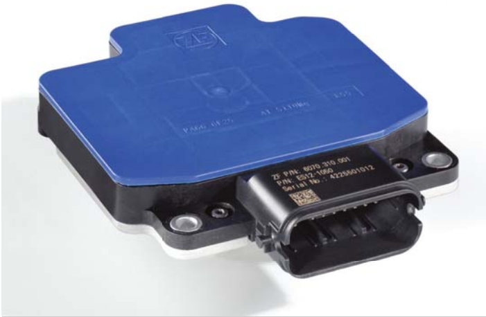
To make sure that everything operates properly and economically, ZF offers their EST 54 Electronic Control System that monitors and directs the electric drive system. ZF.
