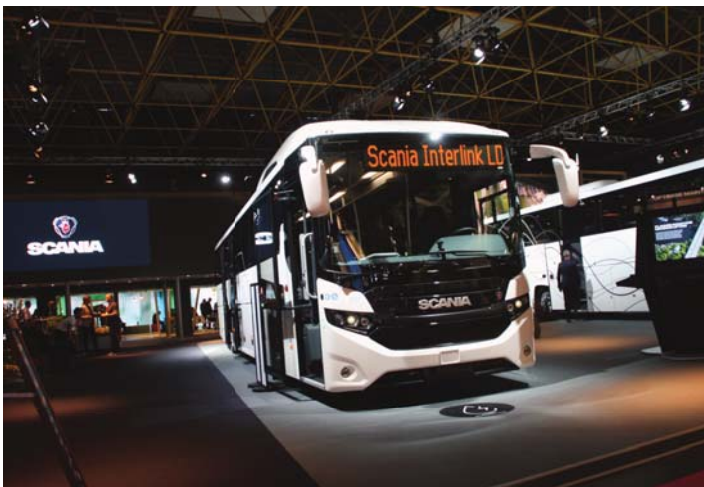
Scania showed off their Interlink LD (low decker) transit. It is available in different lengths form 12 to 15 meters and in a multitude of power options.
