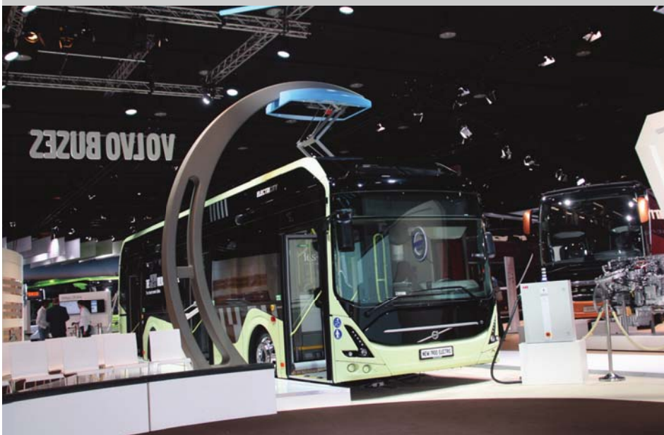
Volvo showed off the latest version of its 12-meter 7900 electric transit bus. It now offers an extended range and more charging options. It can be charged at the end of the line with its overhead charging equipment or with a standard charging cable.
