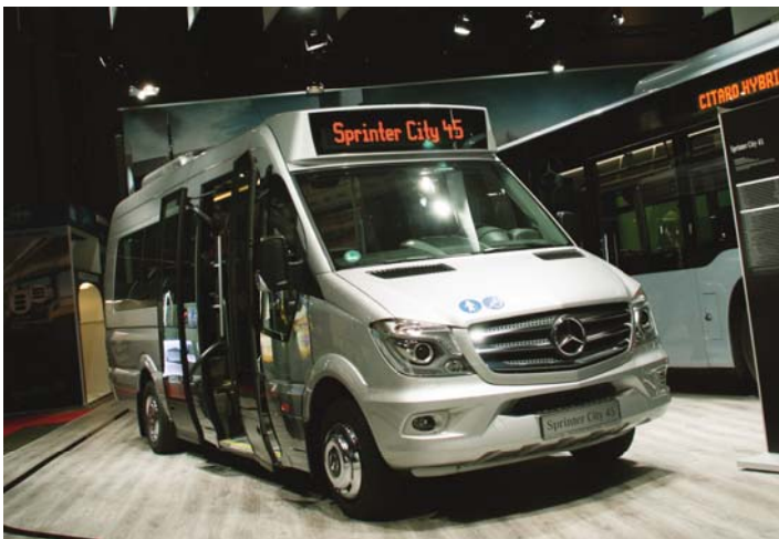
One of the new vehicles shown by Mercedes-Benz was this Sprinter 45 Minibus. Based on the economical Sprinter, it offers 13 seats at the rear plus room for nine standees or wheelchair space in the low-floor area.
