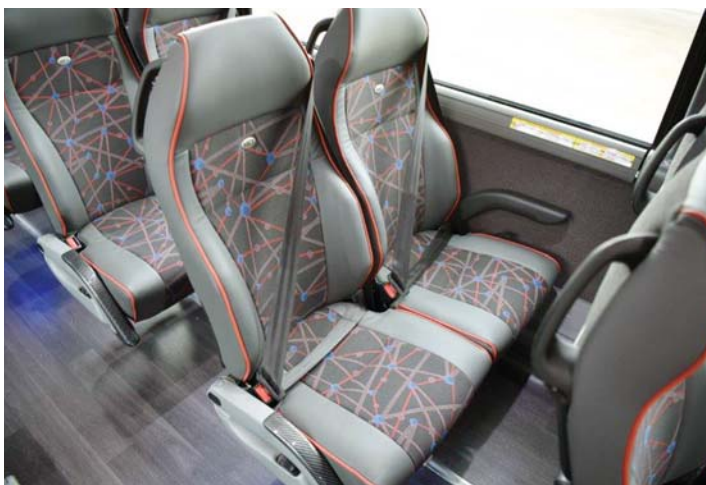
Putting seats with seat belts on a new coach is not that difficult once the engineering work is done and components are modified. However, retrofitting seats with seat belts on an older coach can be a costly uphill battle. This photo shows Kiel seats on the MCI J4500 displayed at the recent UMA Expo. MCI.
