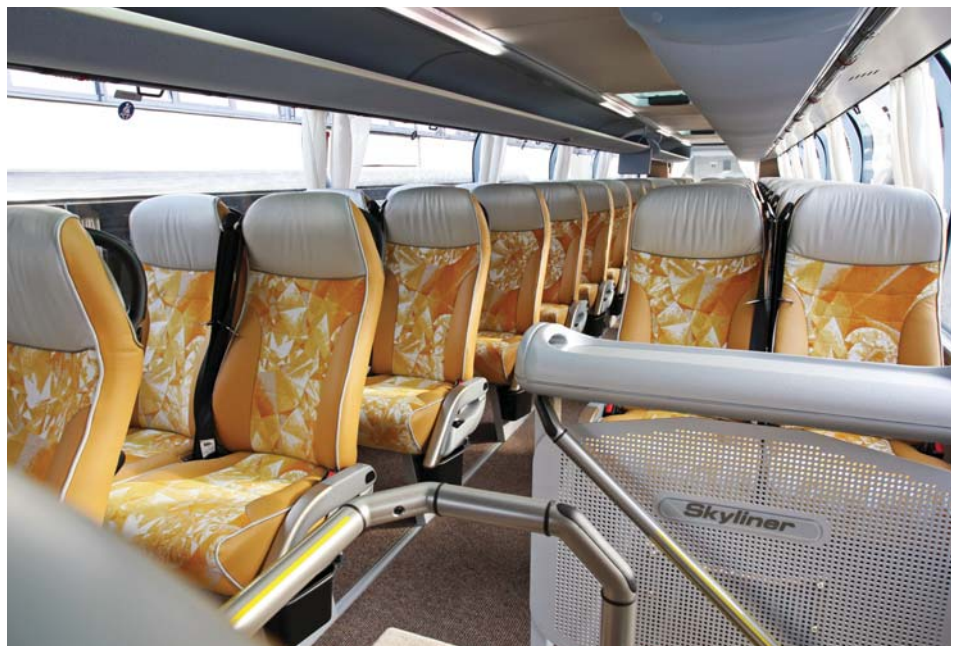
The Europeans started moving to seat belts in the 1990s. Some of their early regulations differentiated between seats with compartmentalization and those without. Shown here is the interior of a Neoplan double-deck Skyliner equipped with three-point seat belts. NEOPLAN.
