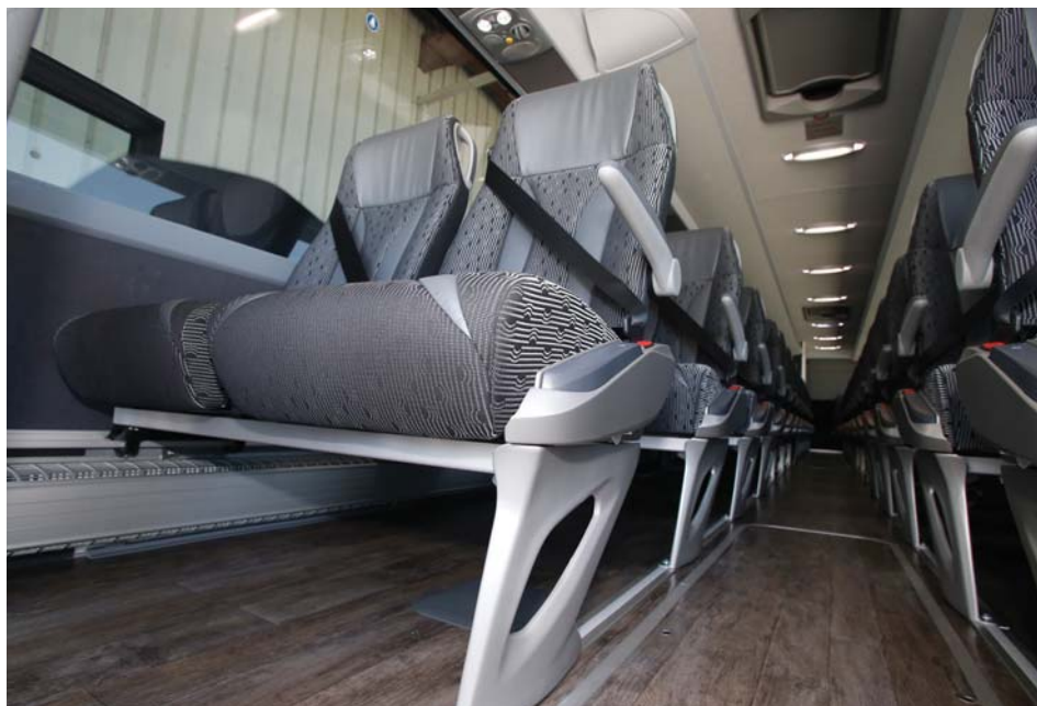
While most passengers do not look down here, this is the area of concern when installing seats with seat belts. In many cases the seat itself has to be strengthened as well as seat tracks and some of the understructure. This photo shows seats on a new Setra coach. MCI.
