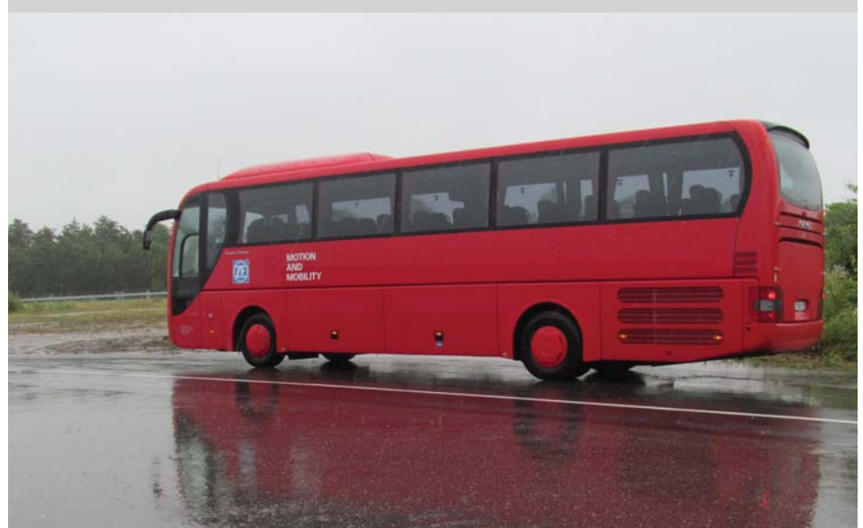
With a length of 12 meters, two axles, two doors and an AS Tronic transmission, the M.A.N. Lion's coach was fairly typical of a standard European coach. It handled very well on the test track and did very well with acceleration and braking. It was equipped with ZF's PCV shock absorbers with steps and gradients that keep the body stable at all speeds. NBT.
