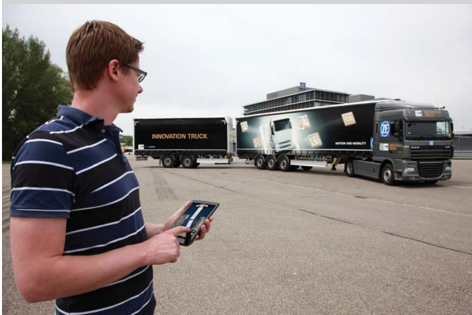
The ZF Innovation Truck is powered by a TraXon hybrid drive. Upon reaching its destination, the driver simply steps out of the cab and parks the truck using a tablet with Bluetooth and an App. It was absolutely impressive to watch that tractor back up by itself with both a semitrailer and a trailer hooked behind. ZF.
