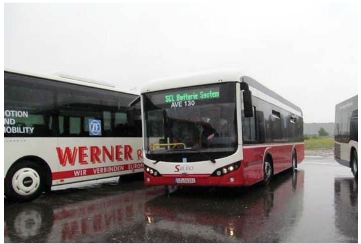
The Bozankaya Sileo model from Turkey was an all-electric, battery-powered bus. It used the ZF AVE 130 low-floor axles with built-in electric motors. It had three passenger doors and a standard transit interior. NBT.
