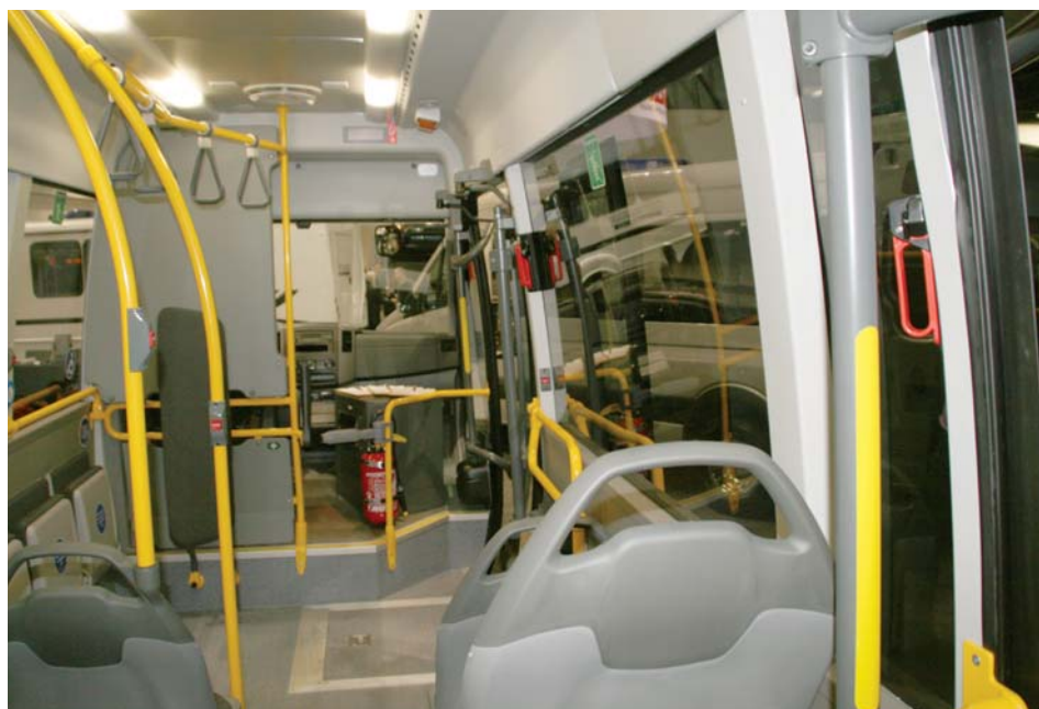
Another interesting bus on display was the two-door Sprinter Citybus 65 from Dortmund. Based on the basic Sprinter design, it offers a small transit interior plus paratransit capability. This photo looks from the seats near the rear door on the right towards the front of the bus that has a ramp and wheelchair tie down locations.
