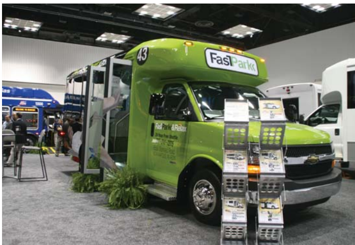
While there were fewer cutaways on the show floor this year, they continued to dominate the show. This example is an ELDorado-National Aerotech on a Chevy chassis with an airporter interior.
