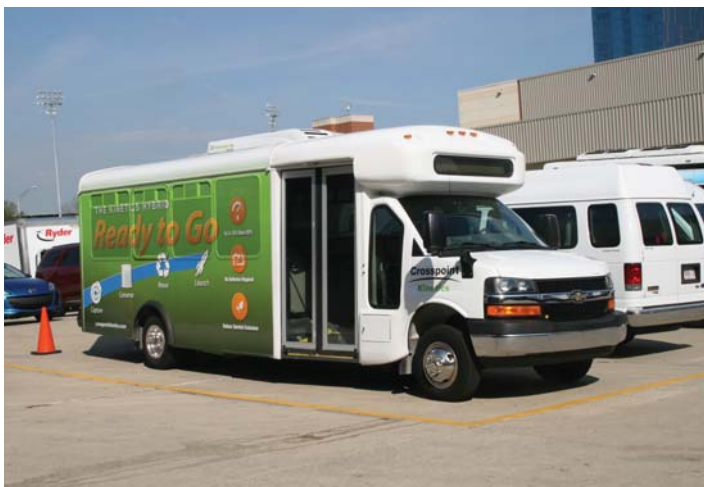
Among their several vehicles available for rides in back of the convention center was this bus on a Chevy chassis equipped with the Crosspoint Kinetics electric hybrid power system.
