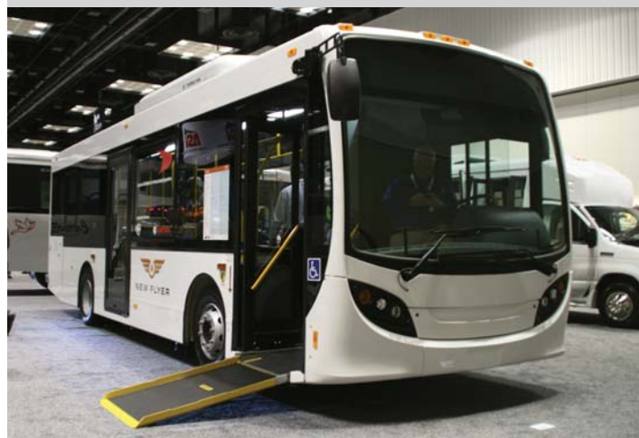
This two-door low-floor New Flyer Midi transit bus was displayed in the Ameritrans booth. It offered a ramp at the front door for wheelchairs.
