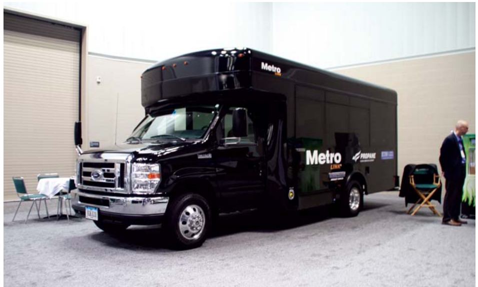
This Winnebago Metro Link was on display in the Propane Education and Research Council booth. Icom North America provided their JTG II Bi-Fuel Liquid Propane Autogas Injection System for the power. One of the best features of the system is that it will switch automatically to gas for longer trips.
