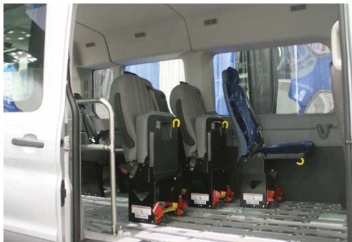
Fenton Mobility had a Ford Transit modified with their Abilitrax system that allows seats to be moved around or removed to reconfigure the interior for different needs as required.
