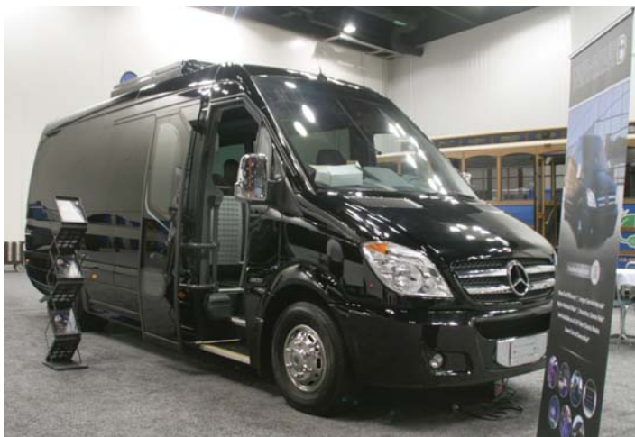
Dur-A-Bus showed this Sprinter that had been modified from the original design with a larger windshield and larger passenger windows. The interior featured colored leather seats.
