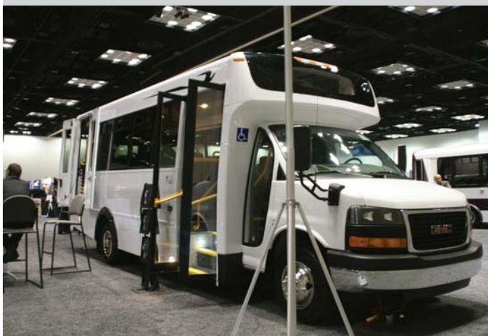
Girardin from Drummondville, Quebec had their G5 special needs Micro Bird bus on display. Note the wheelchair lift at curbside in the rear.
